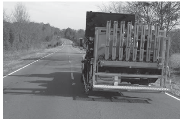
The automated pavement marker placement system fits on a truck and eliminates the need for a worker riding under the truck to apply markers by hand.
