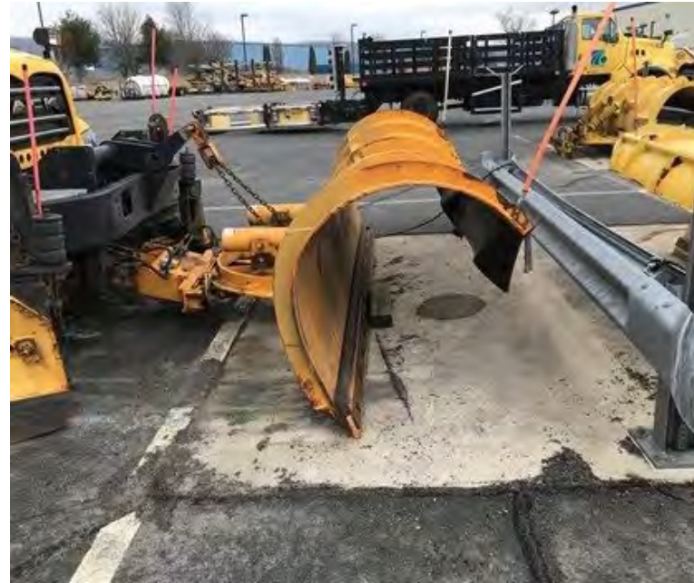
Retrofitted plows have a smaller curve height. Source: PennDOT
