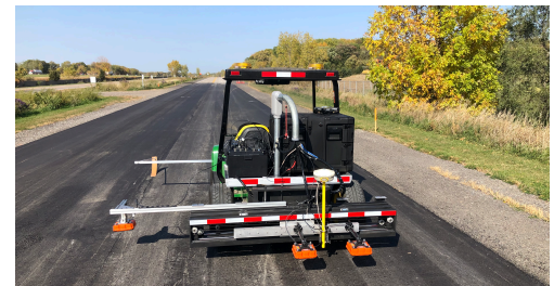
Below: MnDOT tests mounting DPS on a utility vehicle. Source: MnDOT.
