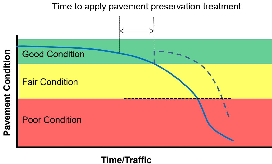
**Figure 3. Concept for proper time to place a pavement preservation treatment.**
