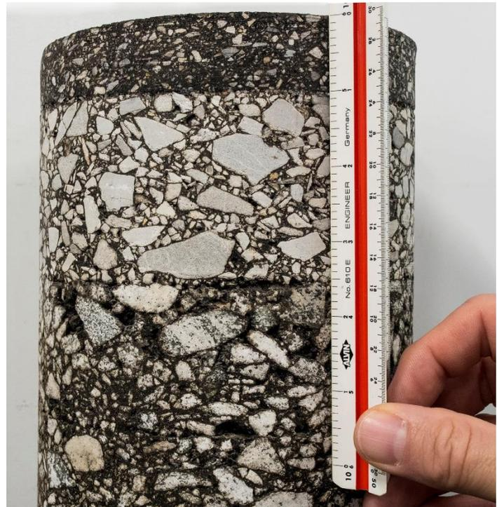
Figure 1. Picture of a thin asphalt overlay.
