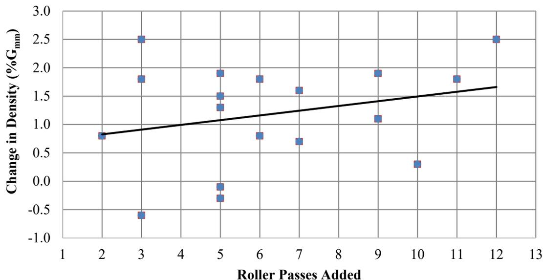
**Figure 1. Change in Density with Added Passes.**
