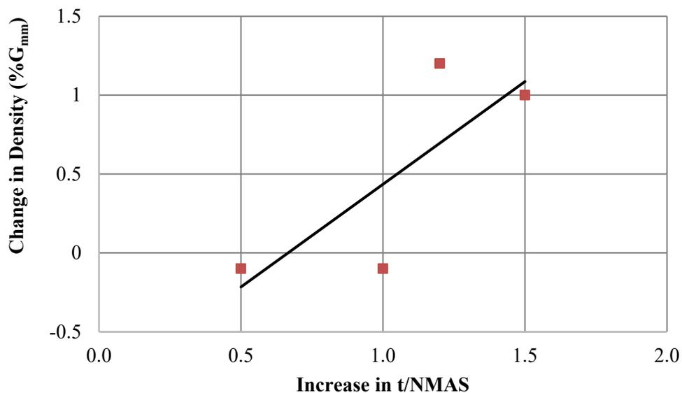
**Figure 2. Change in Density with t/NMAS Increase**
