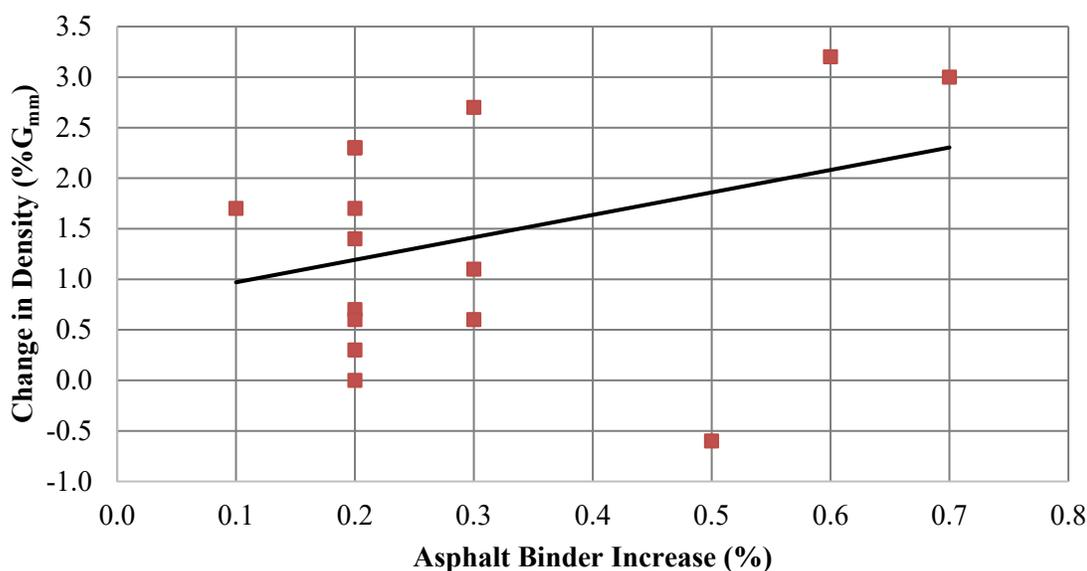
**Figure 3. Change in Density with Increase in Asphalt Binder.**
