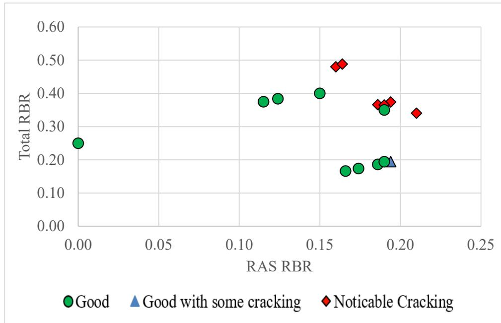
Figure 10. RAS and RAP RBR Levels with Pavement Performance Indicated.
