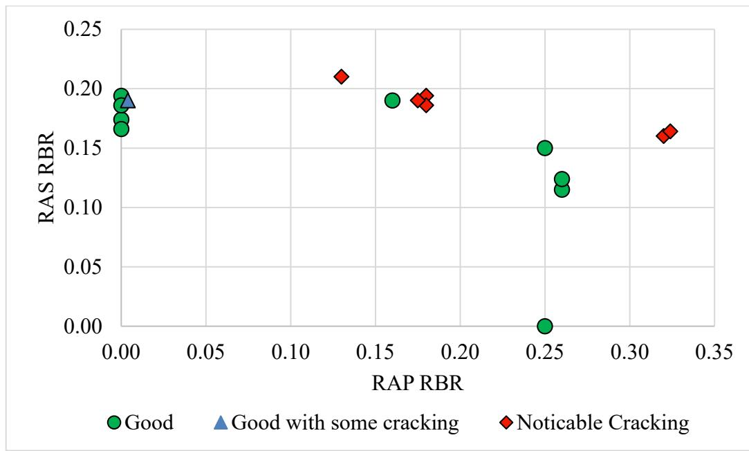
Figure 9. RAS and RAP RBR Levels with Pavement Performance Indicated.
