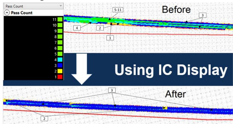
Figure 4. Example of improved roller pass consistency when using IC. [Source: TPF-5(128) Study - Indiana Site]
