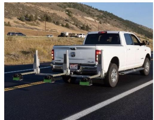
Figure 6. Truck-mounted DPS equipment. (Source: ESS, 2023)
