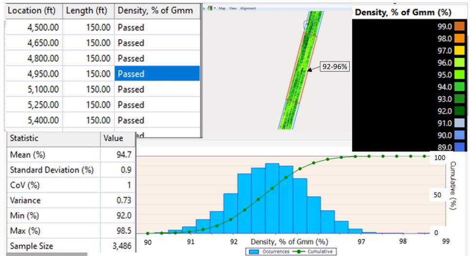
Figure 7. Statistical analysis of data by subplot using Veta. (Source: MnDOT, 2024)
