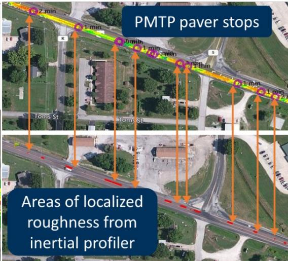
Figure 10. Comparing PMTP paver stops with areas of localized roughness. (Source: The Transtec Group, 2017)
