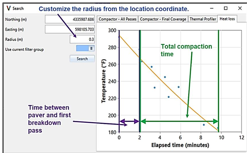
Figure 11. The search tool heat loss curves in Veta. (Source: The Transtec Group, 2022)
