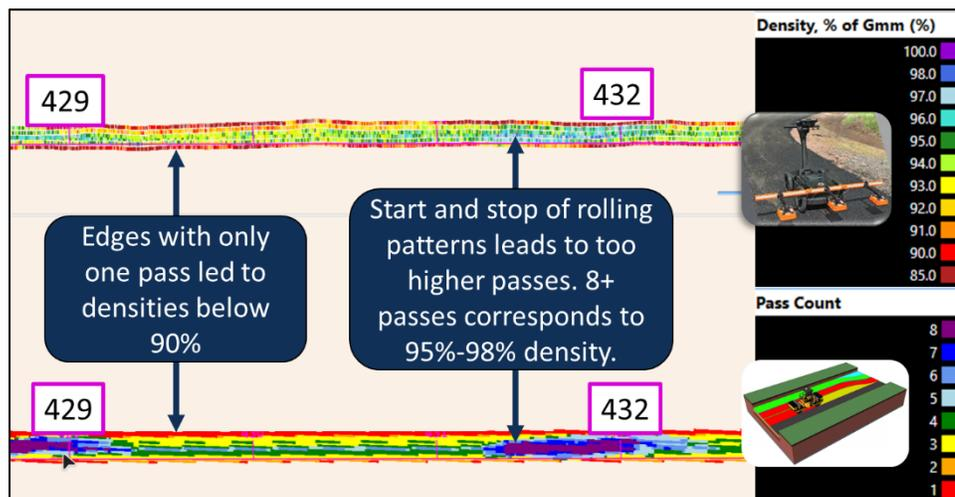
Figure 8. Comparing IC pass count data with DPS estimated density. (Source: ISIC, 2022)
