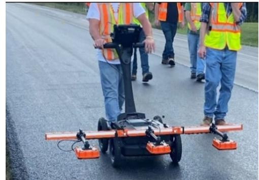
Figure 5. DPS equipment using pushcart. (Source: Gilliland, 2022)
