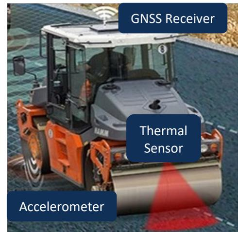
Figure 3. IC roller for asphalt compaction. (Source: Adapted from HAMM)
