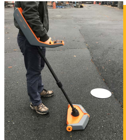
Image Source: FHWA Pulse Induction Technology Device
