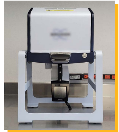
Image Source: FHWA Handheld X-Ray Fluorescence Device
