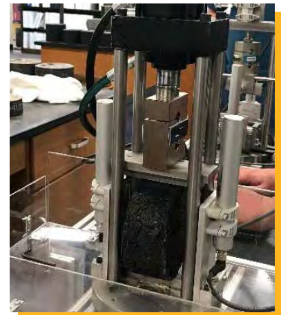
Image Source: FHWA Load Frame performing Ideal-CT
