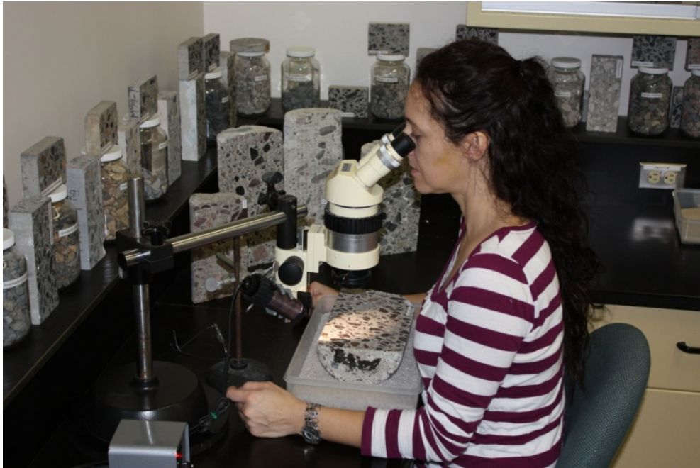
Figure 3 : Examination of the polished concrete section under the stereomicroscope for the determination of the Damage Rating Index.
