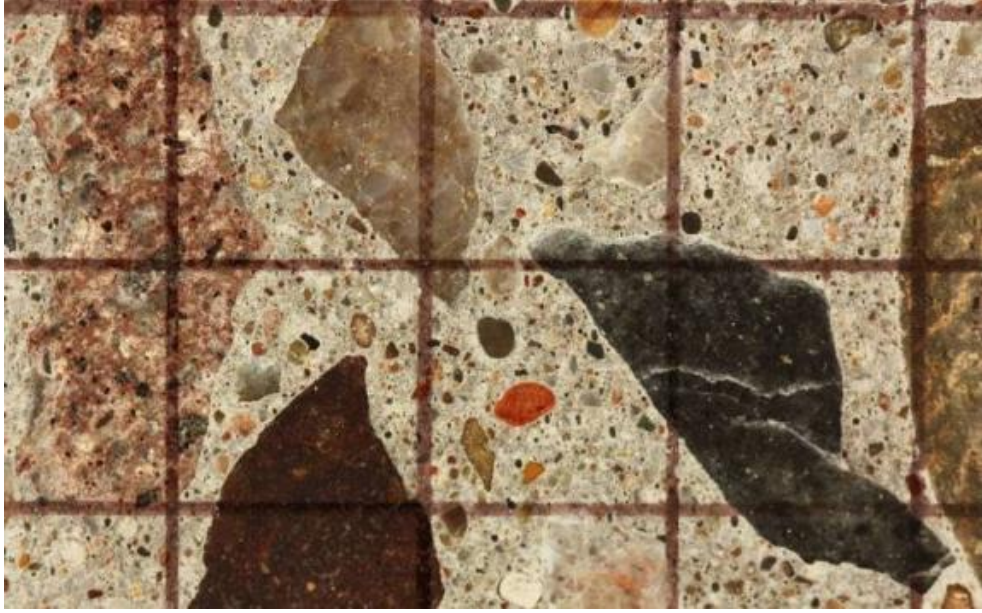
Figure 2 : One cm by one cm grid drawn at the surface of the polished concrete section for petrographic examination using the DRI method.
