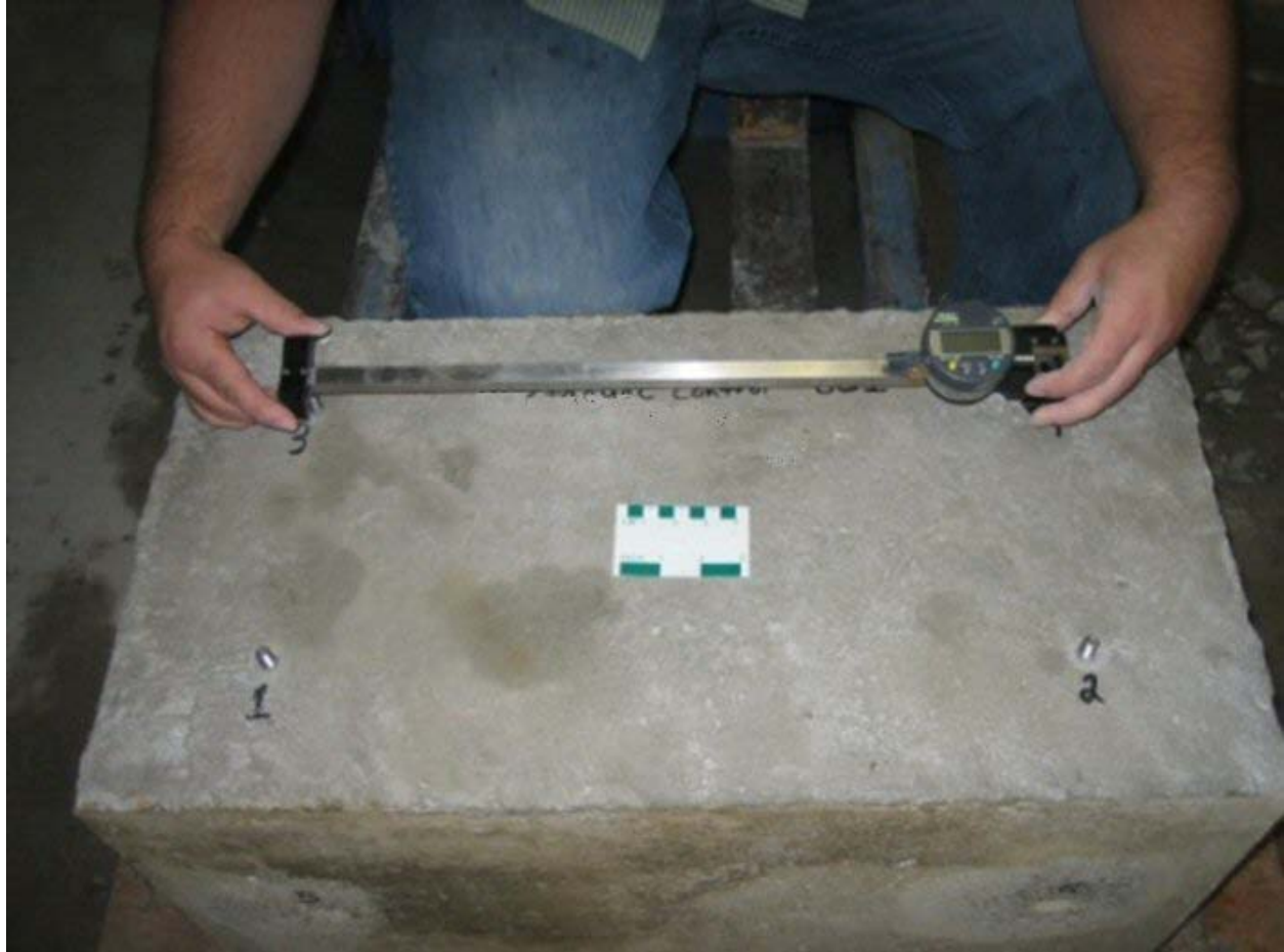
Figure 8. Length-Change Measurements Using a Demec-Type Gauge
