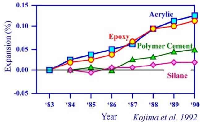
This graph shows data from the Hanshin Expressway in Japan. The graph shows that the application of silane effectively reduced ASR-induced expansion.
