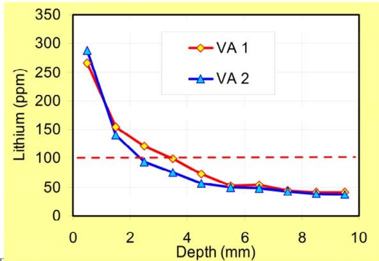
This graph shows the lithium profiles measured on cores extracted from a highway barrier that was vacuum impregnated overnight (the longest and most aggressive vacuum application within this field trial). Once again, the results were not very positive. Despite the significant resources used to attempt to achieve maximum lithium penetration using a long-term vacuum treatment, lithium was only found to be above the threshold value in the outer 2 to 4 mm of the barrier.
