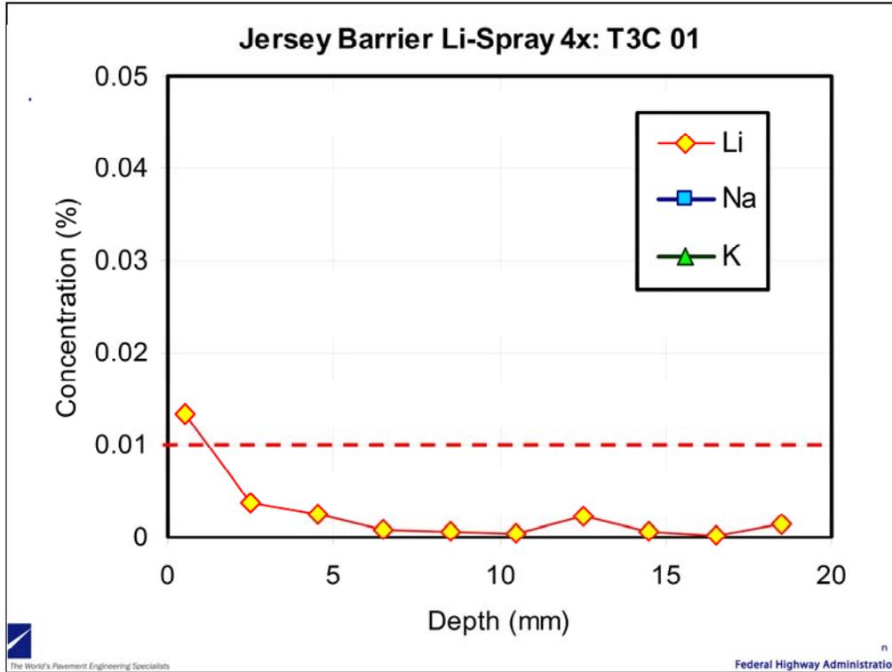
This graph shows the measured lithium profile from a core extracted from a barrier that was treated topically with lithium nitrate four times. Once again, the results are not encouraging. Lithium only was measured to be above the threshold value of 0.01 percent (by total mass) in the outer 2 mm or so.
