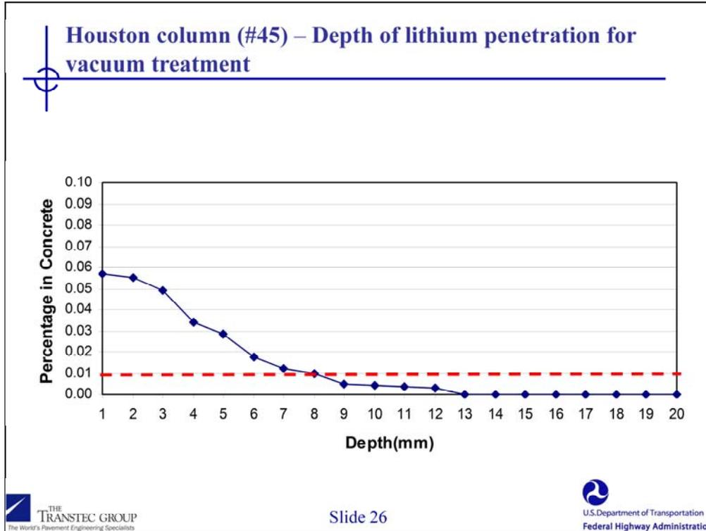
This graph shows the results of the vacuum application of lithium nitrate to an ASR-affected column in Houston, TX. The contractor hired for this field trial had previous experience with vacuum impregnation for repair applications, including the application of lithium nitrate to ASR-affected concrete.
