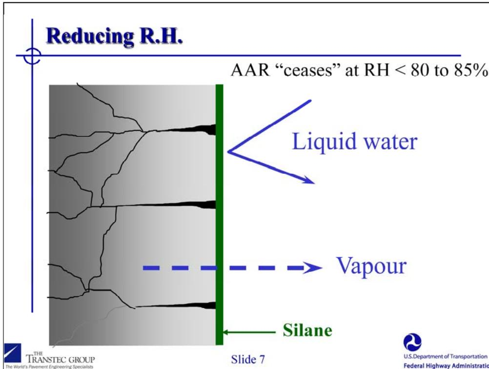
In some cases, it is not possible to improve drainage of water away from an ASR-affected element. In such instances, the application of breathable coatings, such as silanes, may prove helpful. Products such as silanes are effective in preventing liquid water from entering the concrete, while still allowing internal vapor to escape.
