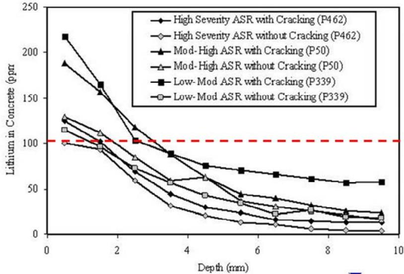
This graph shows the depth of penetration of lithium that was measured in various test sections in the Idaho pavement. The data include the results for pavements with all three degrees of distress (low, moderate, and high), and for each of these sections, data are shown from cores extracted through cracks and away from cracks.
