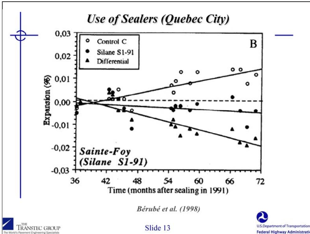
Along with the reduced internal humidity came a reduction in the long-term expansion of the silane-treated barriers. In fact, after six years, the treated barriers had actually exhibited shrinkage, whereas the untreated barriers continued to expand during the monitoring period.
