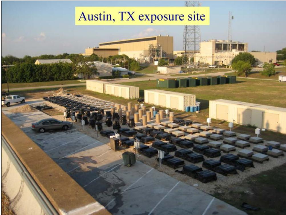
Lastly, there is a relatively new ASR field site in Austin, TX, where the primary focus is on triggering ASR in simulated field structures and then trying to slow down the reaction through various treatments and technologies.
