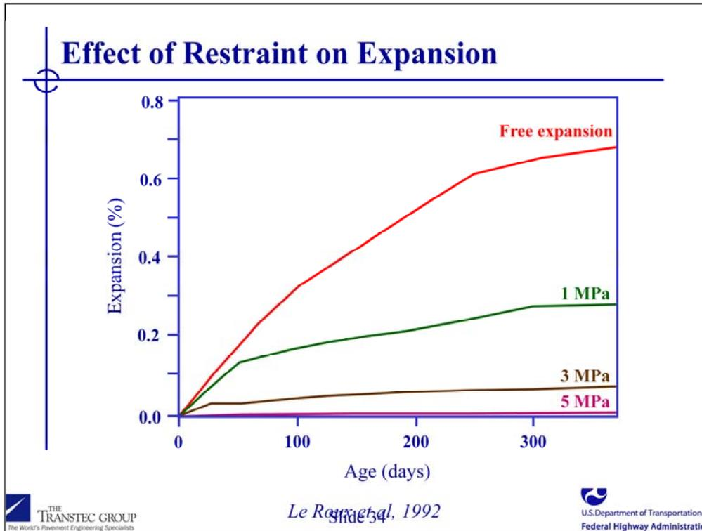
We will now switch gears and discuss some other methods that have been used in the laboratory and/or field to attempt to reduce the future expansion of concrete structures already affected by ASR.
