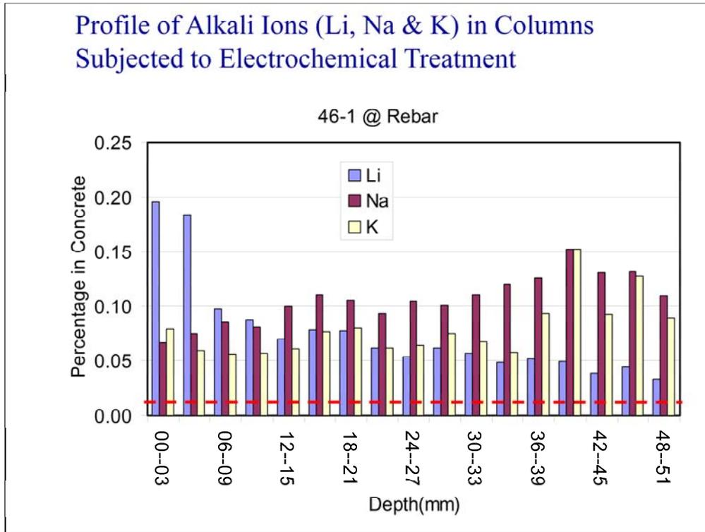
This graph shows the concentration of Li, Na, and K as a function of distance from the face of one of the electrochemically treated columns.
