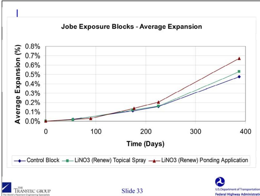
This graph shows the average expansion for the three blocks shown on the last three slides.
