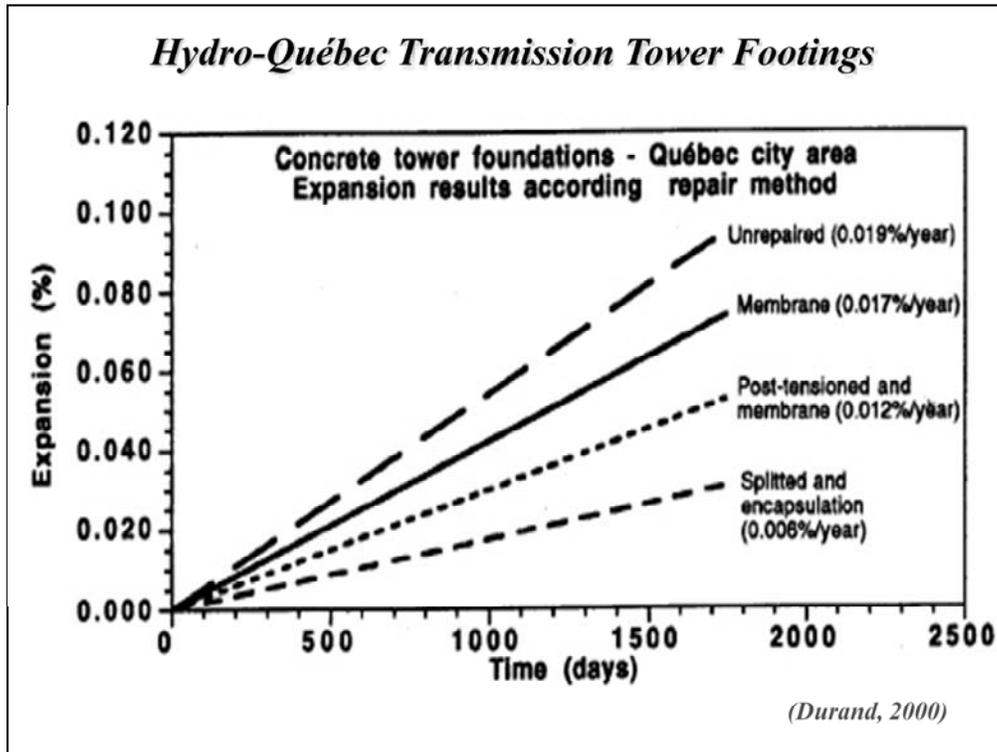
This graph shows the expansion data for the Hydro-Quebec field trials on tower footings. The data shows that all mitigation measures reduced expansion relative to the untreated control footing. The most effective method was found to be the encapsulation of ASR-affected footings with strong, dense, reinforced concrete. Post-tensioning also was found to be a viable means to reduce expansion.
