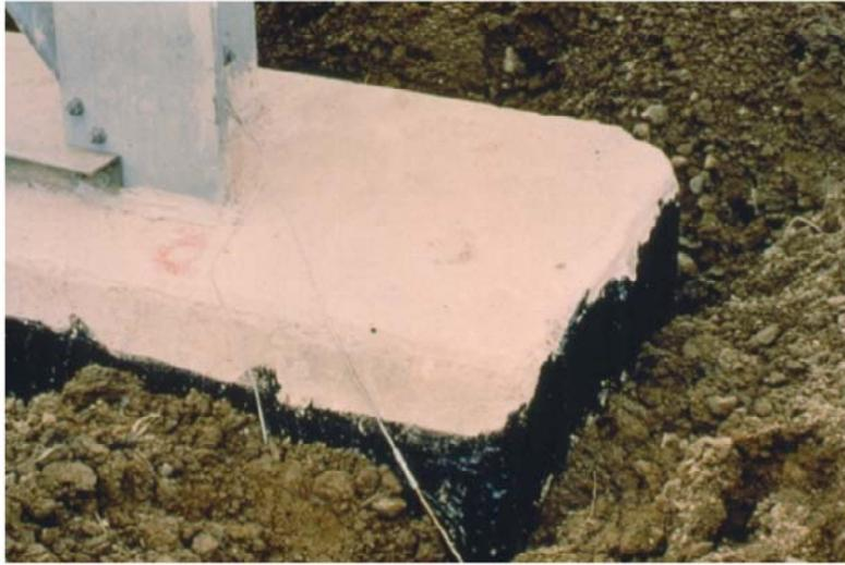
Other footings from the same field trial were enveloped with a water-proofing membrane, with the overall objective of decreasing the availability of water to the ASR-affected concrete.
