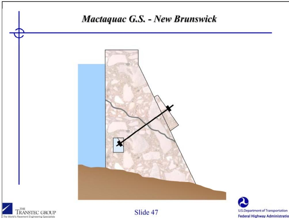
As shown in this depiction, post-tensioning rods were inserted through a dam and were anchored in the interior of the dam and at its downstream face. This repair seems to have adequately addressed the concern regarding the large crack through the dam. However, because of operational difficulties, this dam is slated for replacement in the next 10-20 years.
