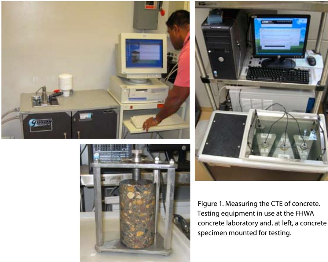
Figure 1. Measuring the CTE of concrete. Testing equipment in use at the FHWA concrete laboratory and, at left, a concrete specimen mounted for testing.
