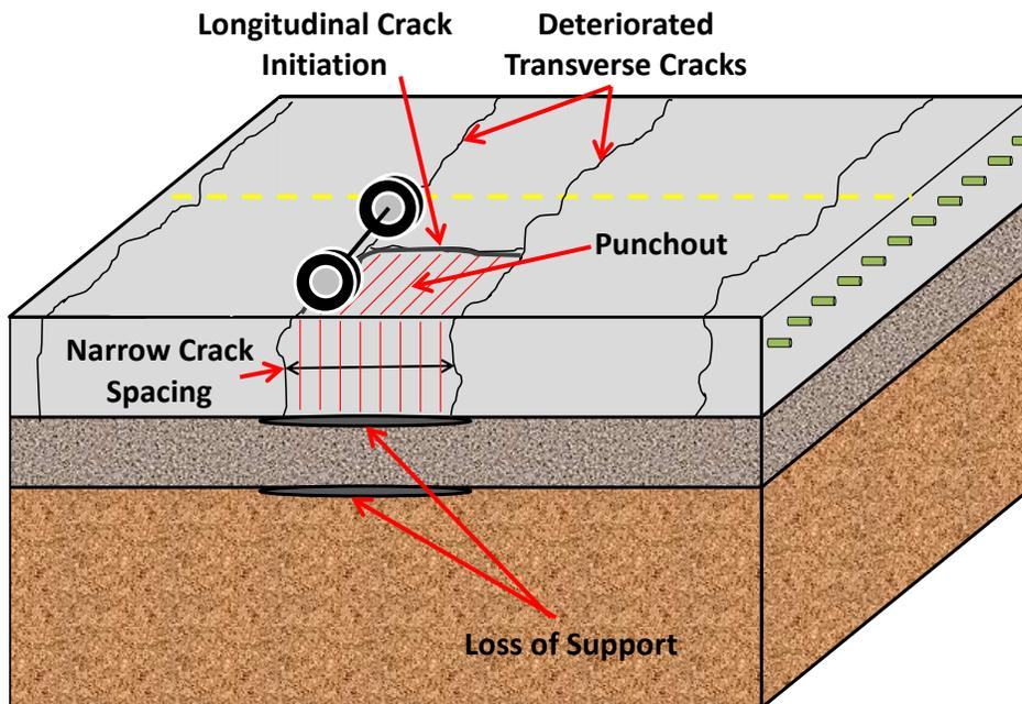
**Figure 1. Schematic of CRCP punchout mechanism.**
