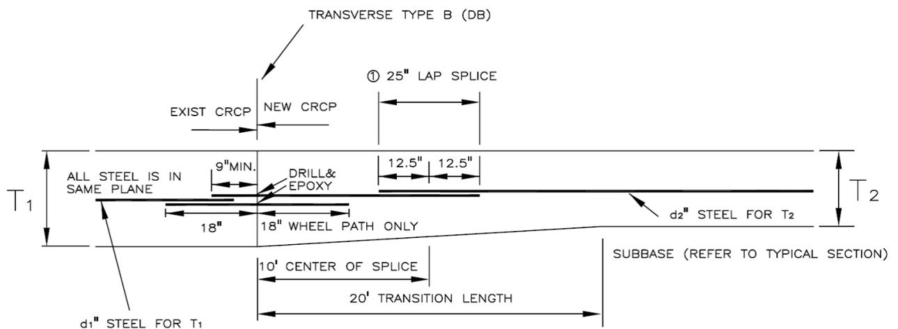
FIGURE 3. Thickness transition detail for CRC pavement.
