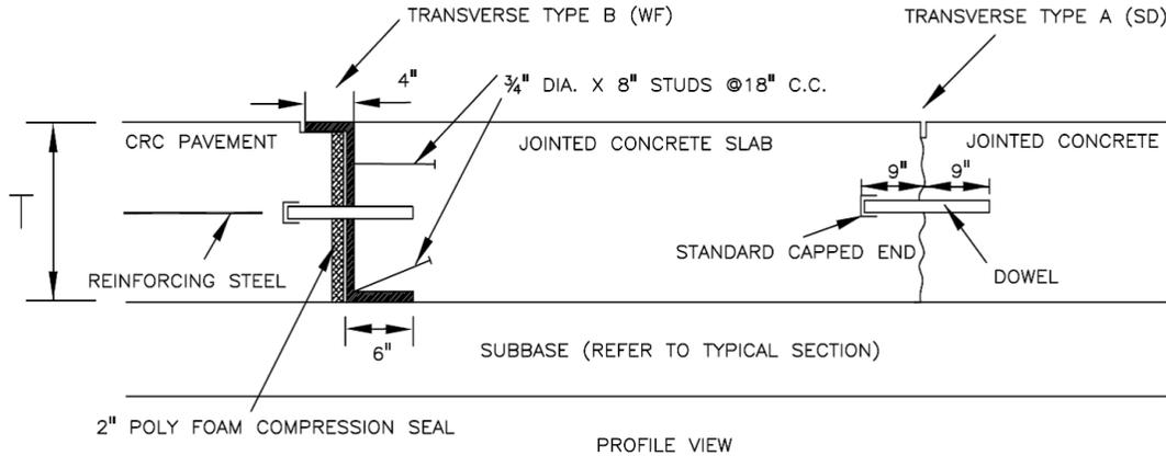
FIGURE 5. Transition details between CRC and JC pavements using a modified wide flange.
