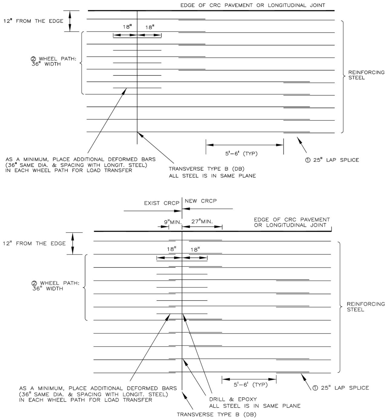
FIGURE 2. Wheel-path reinforcing details of a CRC pavement construction joint. (1 inch = 25.4 mm; 1 ft = 0.305 m)
