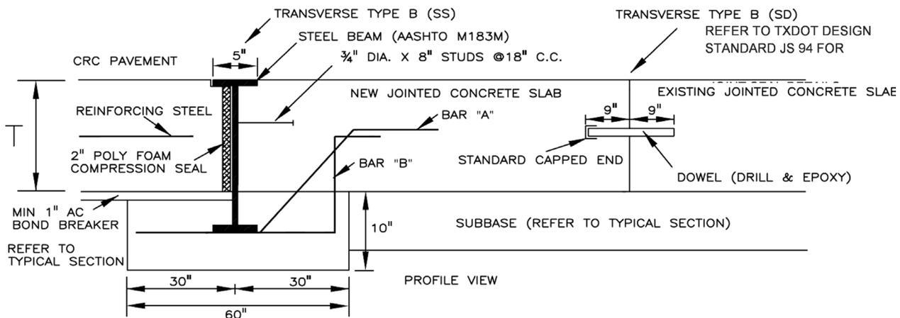
FIGURE 4. Transition details between CRC and JC pavements using a sleeper slab and a wide-flange I-beam.
