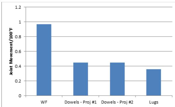
FIGURE 1. Summary of joint movement at different transition joints and sites. (WF = wide flange)
