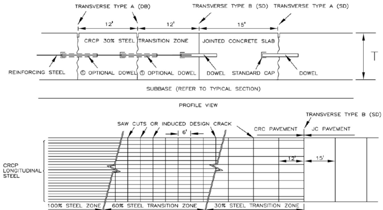
FIGURE 7. Transition between CRC and JC pavements using steel transition and saw cuts.
