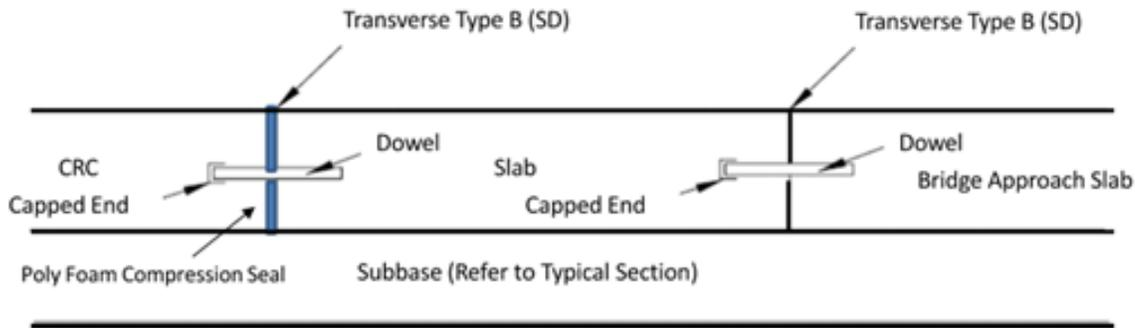
FIGURE 6. Transition detail between CRC and JC pavements using a doweled joint.
