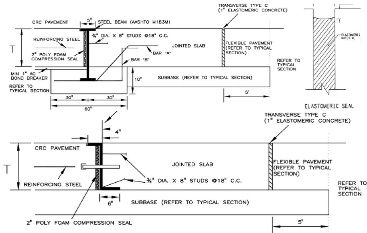
FIGURE 9. Transition between CRC and AC pavements using elastomeric concrete and a JC pavement slab segment.
