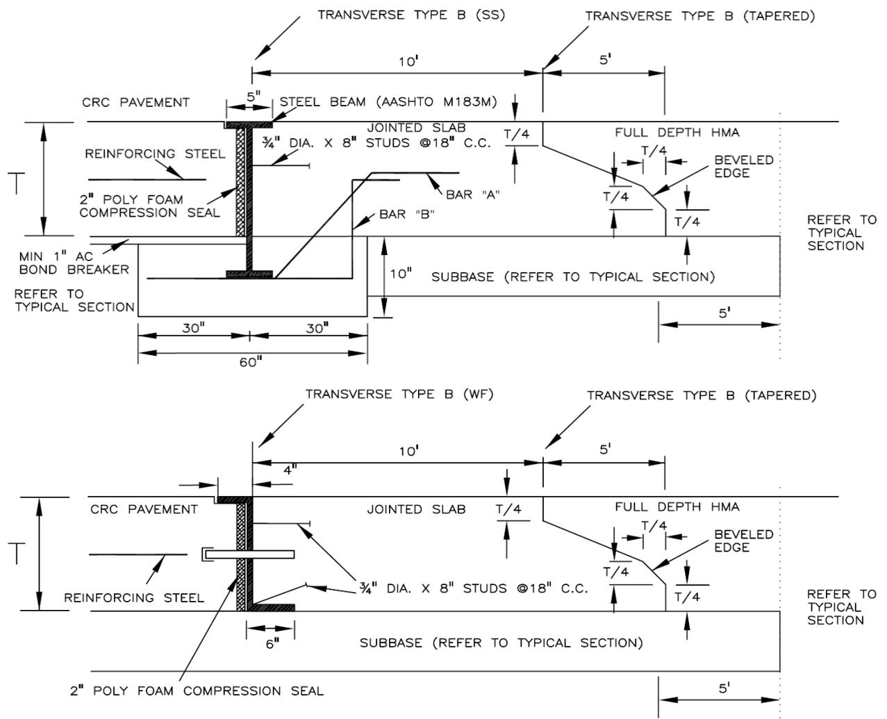
FIGURE 8. Transition between CRC and AC pavements using a tapered slab.
