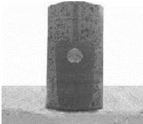
Figure 6. Photo. Bottom slot filled with grout.
