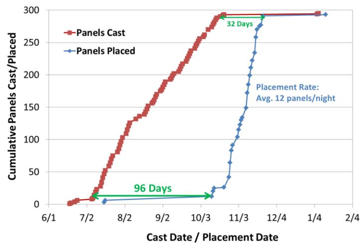
Figure 14. Graph. Panel fabrication and panel installation rates.
