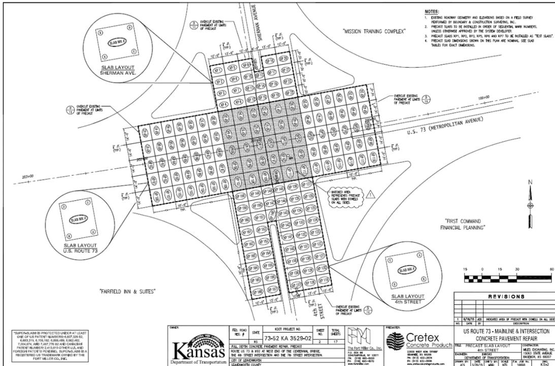
Figure 4. Diagram. Panel layout at the intersection of US 73 and 4th Street.
