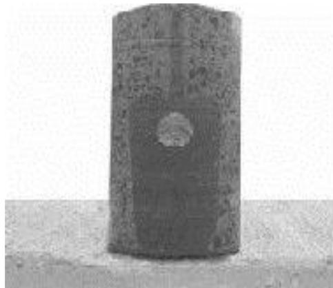
Figure 9. Photo. Bottom slot filled with grout.
