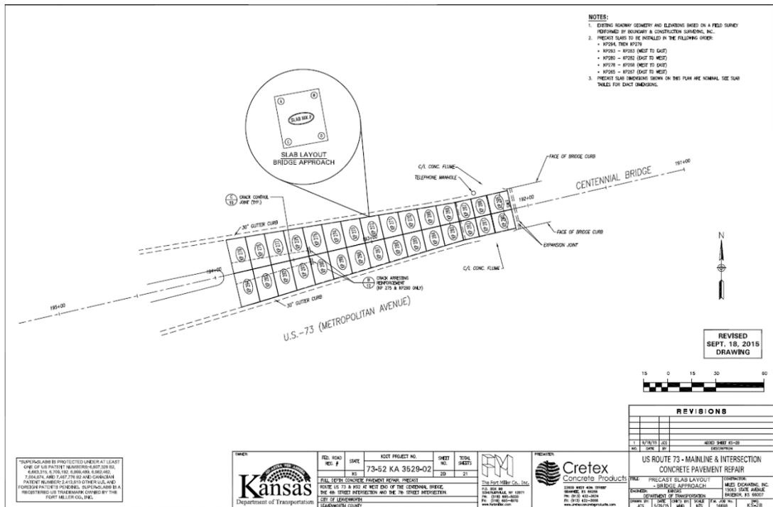
Figure 5. Diagram. Panel layout at the approach to Centennial Bridge.
