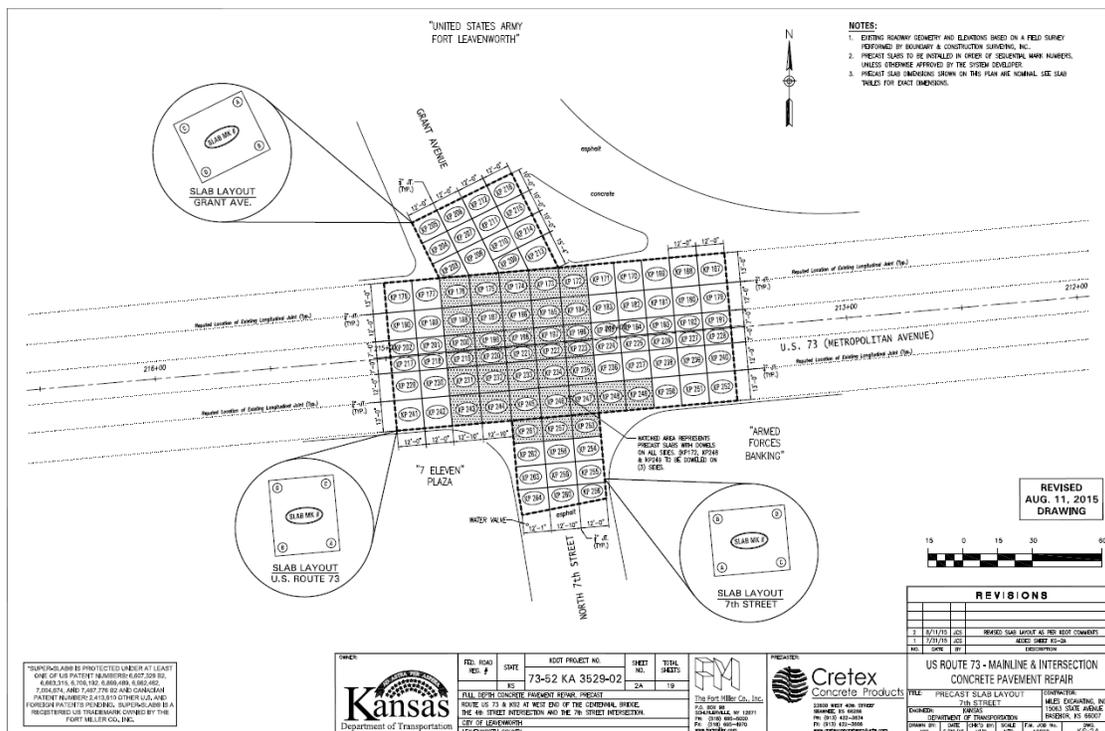
Figure 3. Diagram. Panel layout at the intersection of US 73 and 7th Street.
