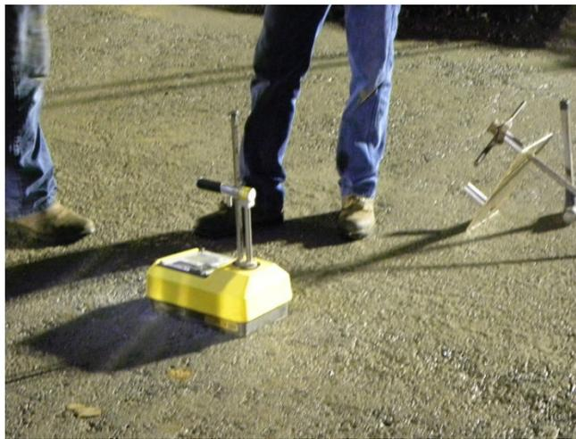
Figure 15. Photo. Base compaction testing using a nuclear gage.
