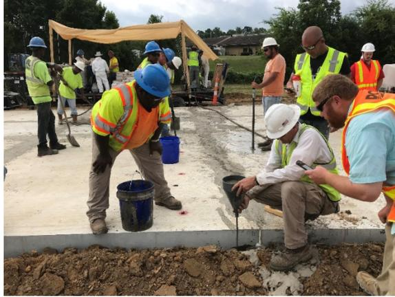
Figure 27. Photo. Efflux testing for the bedding grout.
