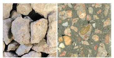
Miras Mamirov, University of Nebraska, used with permission Figure 1. RCA produced from interstate highway pavement (left) and polished sawcut face of RCA concrete showing residual mortar (lighter paste area) on coarse RCA particles with new mortar darker in color (right)
