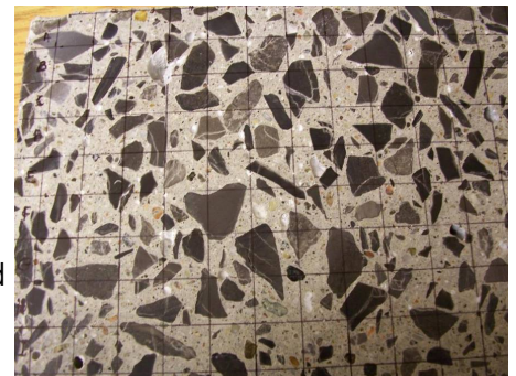
Figure 1. Prepared concrete sample for DRI evaluation.
