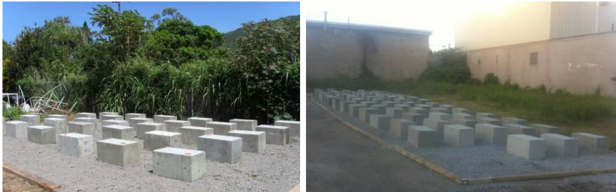
Figure 5. Hawaii DOT and Massachusetts DOT outdoor exposure sites.
