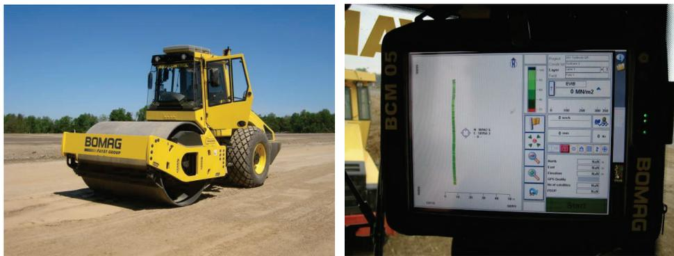
**Figure 17. A single-drum Bomag roller equipped with roller-integrated  $E_{VIB}$  measurement system on-board display units with BCM-05<sup>®</sup> software.**
