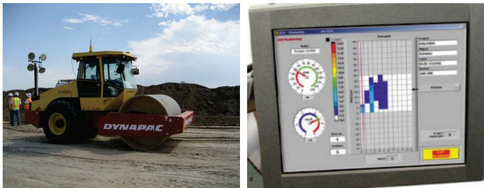
**Figure 19. A single-drum Dynapac roller equipped with roller-integrated CMV measurement system and on-board display unit with DCA<sup>®</sup> software.**
