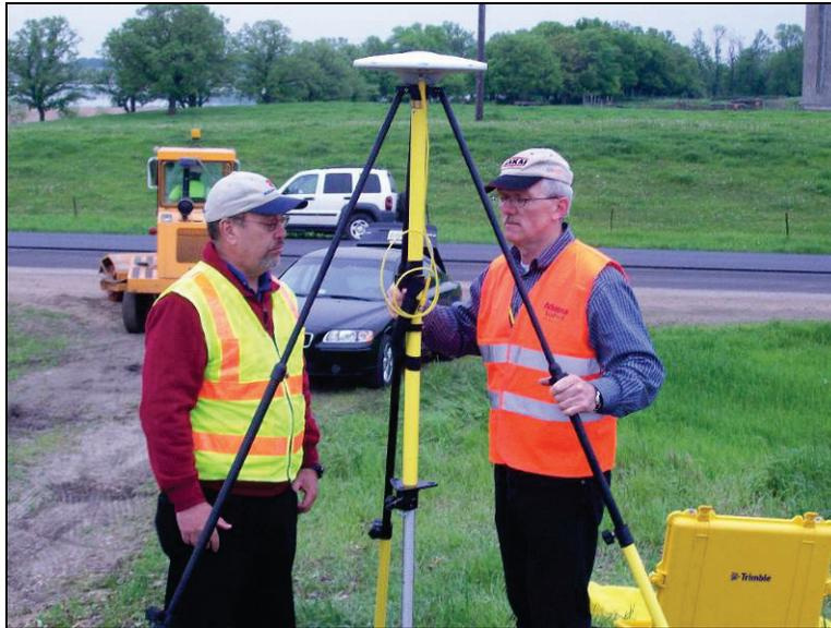
**Figure 13. A Trimble GPS base station (ICPF MnDOT demo).**
