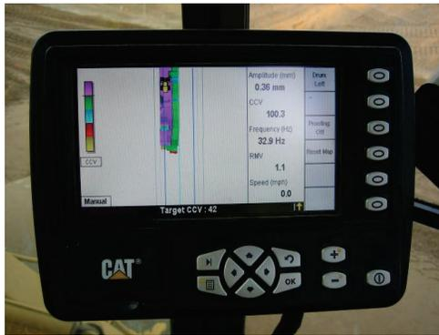
**Figure 18. Caterpillar rollers (padfoot and smooth drum) equipped with roller-integrated MDP and CMV measurement systems on-board display unit with AcuGrade<sup>®</sup> software.**
