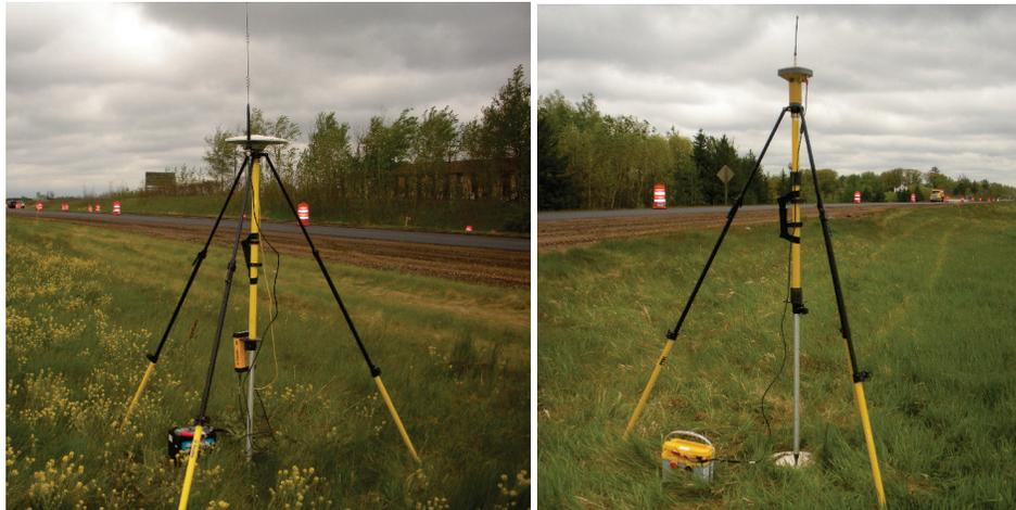
**Figure 192. A Trimble GPS base station (left) and a TopCon GPS base station (ICPF WisDOT demo).**
