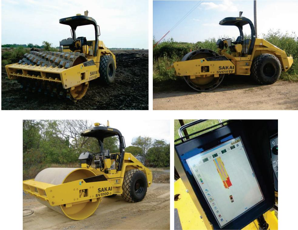
**Figure 20. Sakai rollers (padfoot and smooth drum) equipped with roller-integrated CCV measurement system and on-board display unit with Aithon-MT<sup>®</sup> software.**
