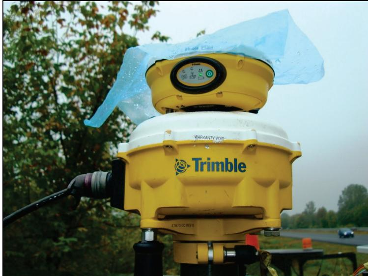
**Figure 194. Validation of roller mounted GPS with a hand-held rover (ICPF VADOT demo).**
