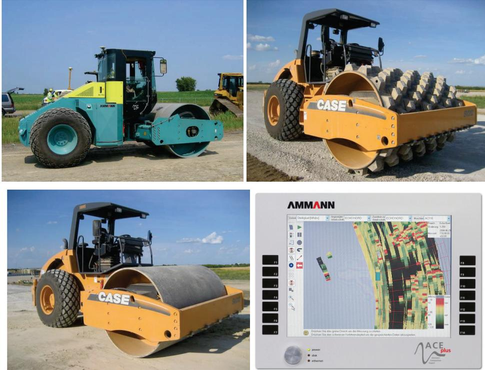
**Figure 16. Ammann and Case rollers (padfoot and smooth drum) equipped with roller-integrated  $k_s$  measurement system on-board display units with ACE-Plus<sup>®</sup> software.**
