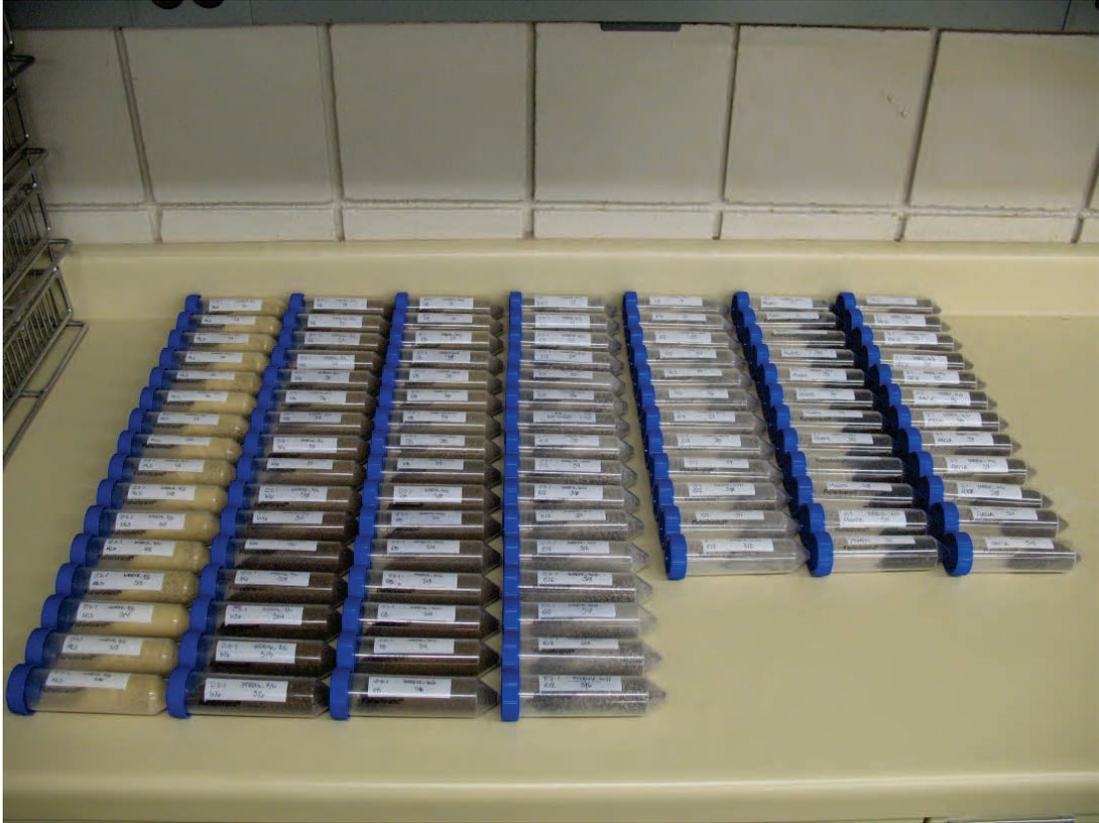
**Figure 14. 55mL vials prepared for leachate tests.**
