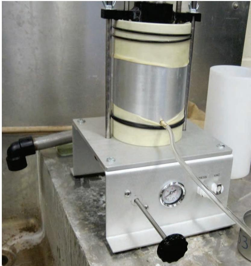
**Figure 43. Laboratory flexible-wall asphalt permeameter.**
