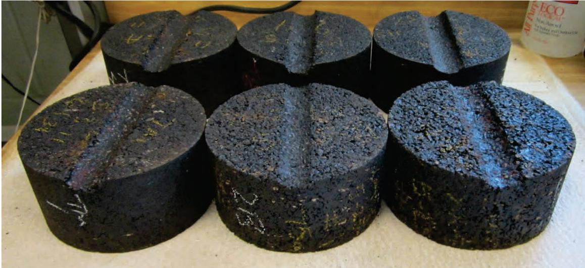
**Figure 45. Example of APA specimens after testing. Clockwise from upper left: Mixture RG-004, T-005, RT-006, RS-003, S-002, and G-001.**
