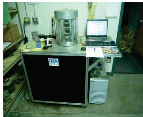
Figure 2: The Interlaken simple performance testing machine
