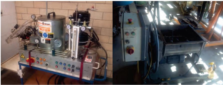
Figure 5: Wirtgen asphalt foamed unit and mixer
