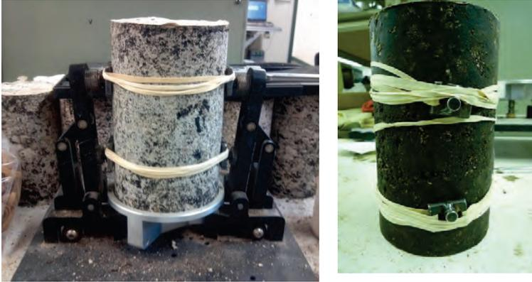
Figure 53: Set points attached to emulsion and foamed asphalt samples with rubber bands
