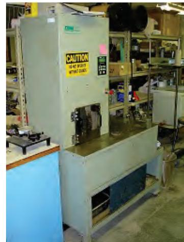
Figure 6: The Superpave gyrotory compactor
