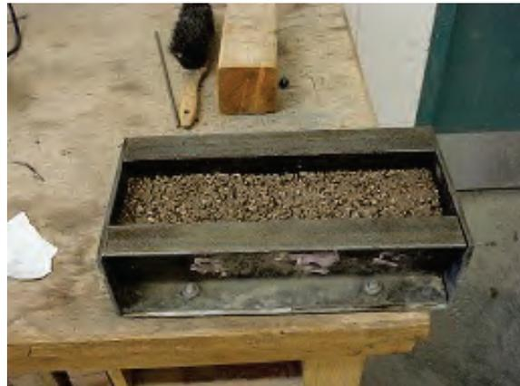
Figure 3: Modulus of rupture sample is shown in mold
