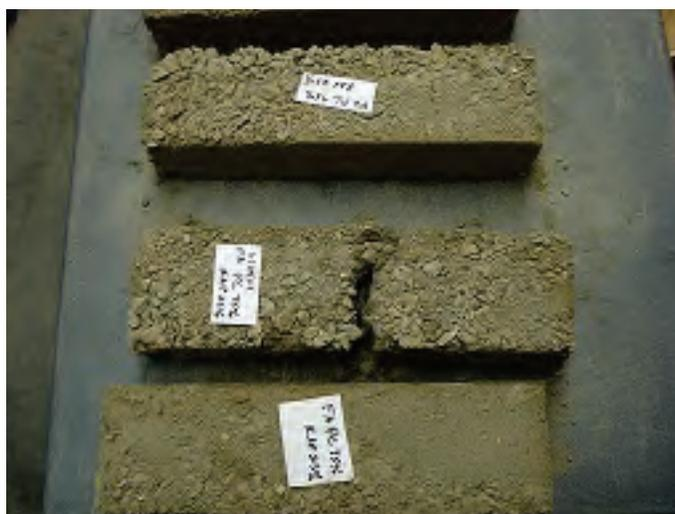
Figure 48: Fly ash modulus of rupture sample broken while handling.
