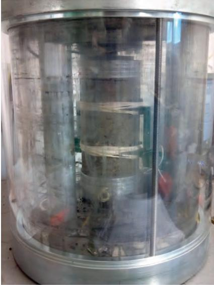
Figure 52: Typical FDR sample in SPT machine ready for dynamic modulus testing
