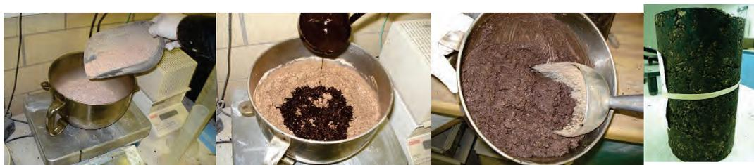
Figure 50: Four of the steps during making of asphalt emulsion test samples
