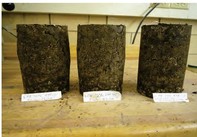
Figure 54: Tested repeated load triaxial samples with the right sample that did not fail.
