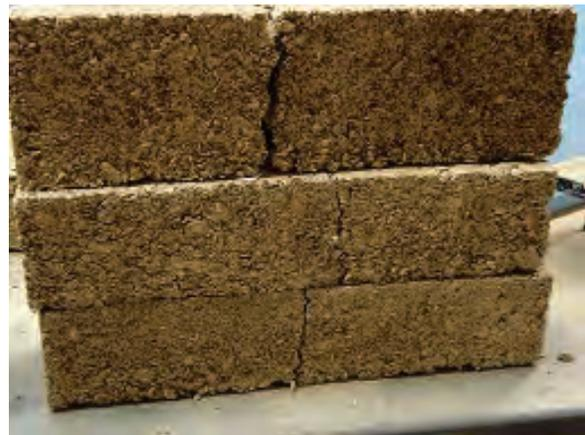
Figure 49: Typical set of modulus of rupture samples.
