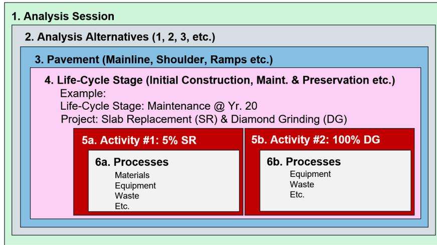
Figure 2-3. Tool structure.
