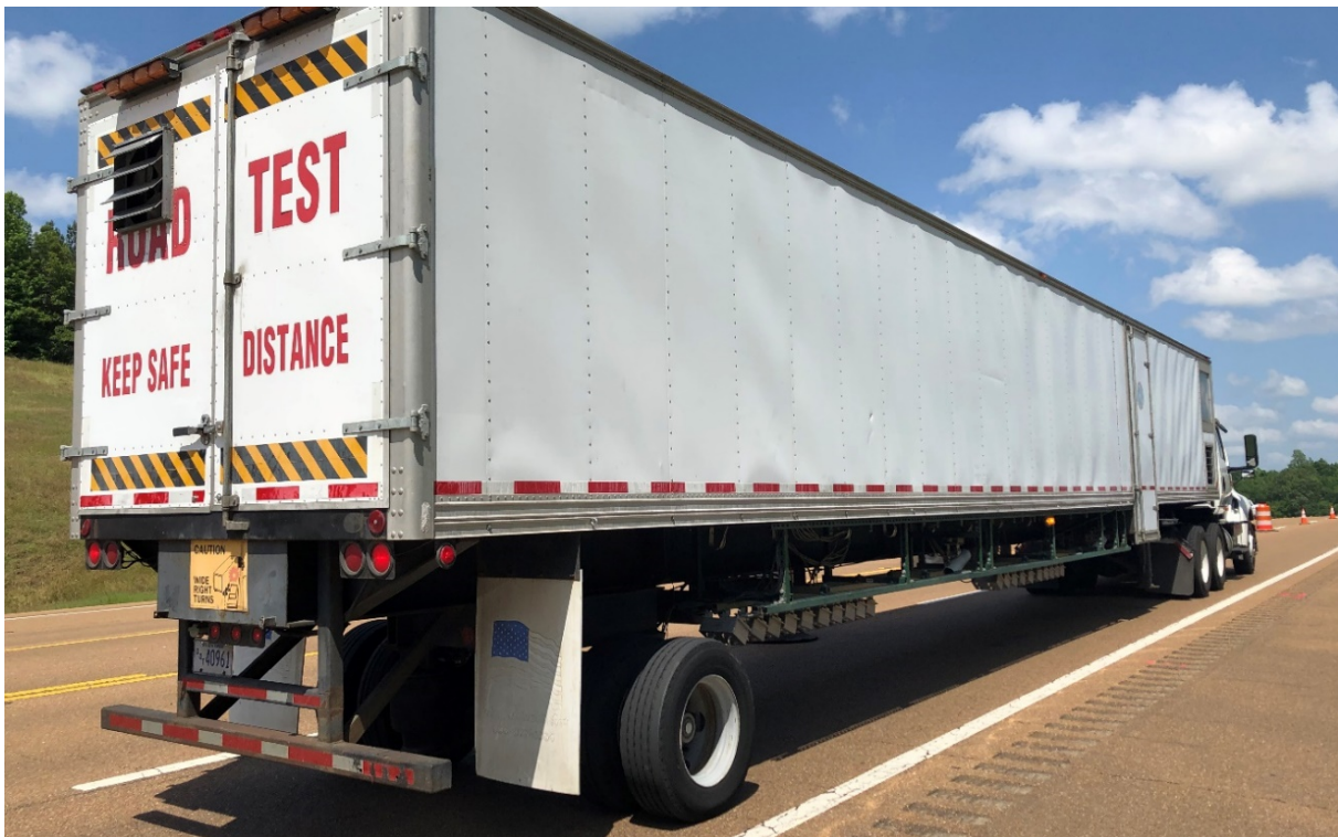
Figure 1. Photo. The RWD measures pavement structural response at highway speeds.
