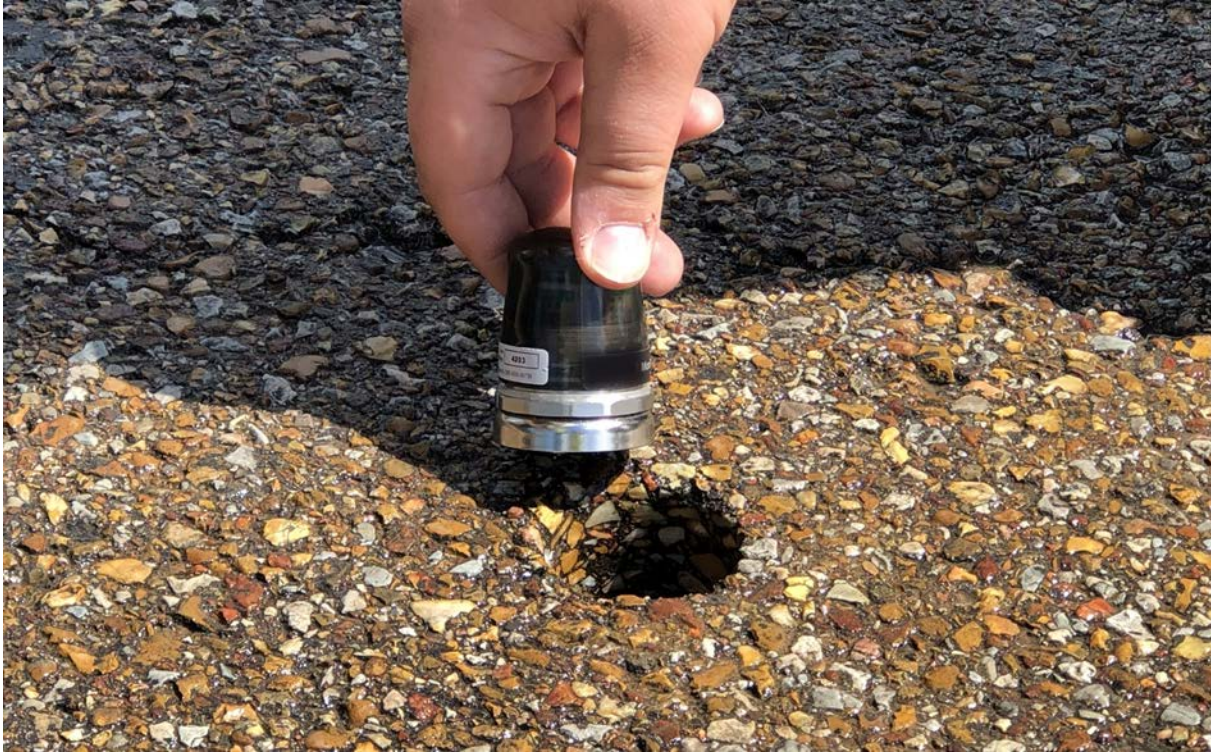
Figure 45. Photo. The accelerometer used for pavement instrumentation.
