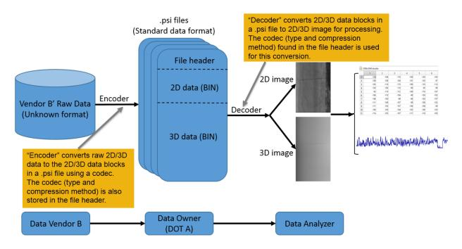
Figure 7. Chart. Preliminary testing of using standard data format.
