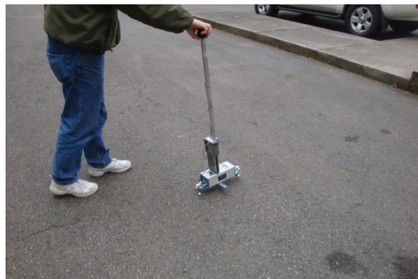
Figure 13. Example of Dipstick® profiler (photo courtesy of WSDOT).
