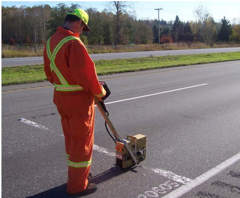
**Figure C-2. Class I roughness survey (BCMoTI 2012).**
