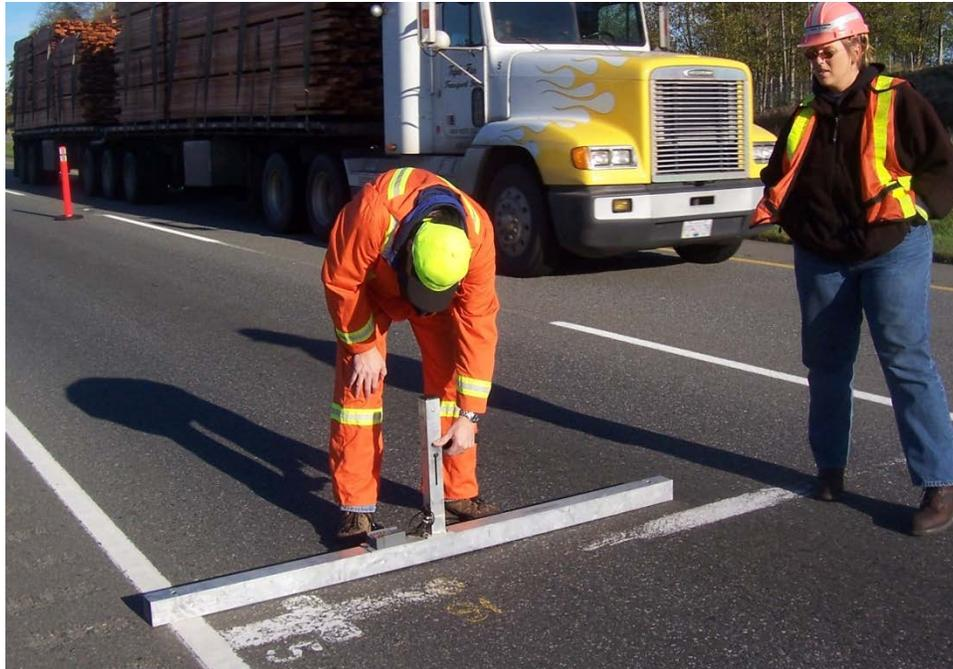
**Figure C-1. Rut depth survey (BCMoTI 2012).**
