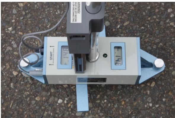
Figure 12. Close-up of Dipstick® profiler (photo courtesy of WSDOT).
