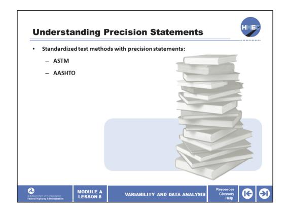
Many standardized test methods, such as those in ASTM and AASHTO, contain precision and bias statements. It is important to understand the meaning of the terms used in these statements. The precision statement provides a measure of how repeatable the test method is. This is very important when it comes to establishing the creditability of a test method. If these numbers tend to be small, the test method is considered to have good precision. The next screen provides an example.
