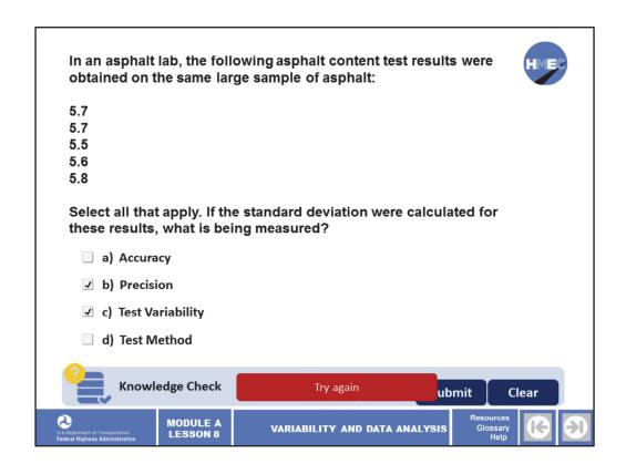
In an asphalt lab, the following asphalt content test results were obtained in the same large sample of asphalt:
