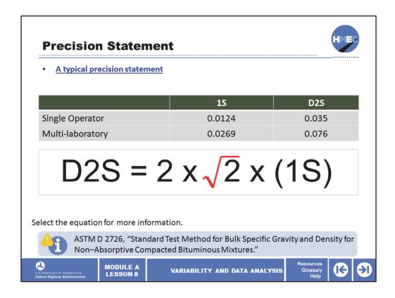
A typical precision statement will have a column with a one-sigma limit (1S) that is used to denote the estimate of the standard deviation of the population of the test method. This limit is usually established for a single operator in the second row, and also for multi–laboratory precision in the third row.
