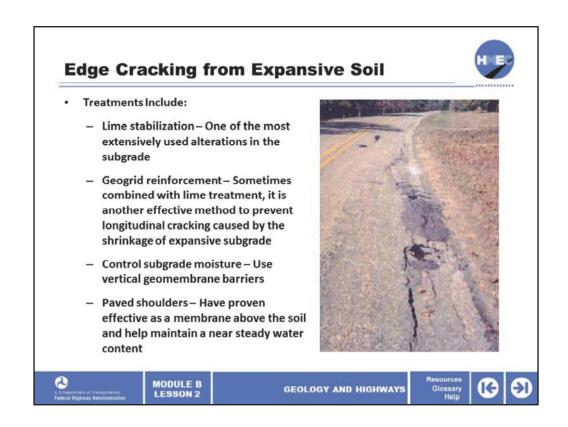
Edge cracking of pavements can be the result of expansive soil in the subgrade. The photograph shows an example of longitudinal cracking from an expansive subgrade on a low-volume road in Texas.
