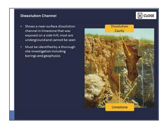
This photograph shows a near-surface dissolution channel in limestone that was exposed on a side-hill. Most are underground and cannot be seen. You can imagine the types of problems these features cause for pavements, piling, and drilled shafts. They must be identified by a thorough site investigation including borings and geophysics.
