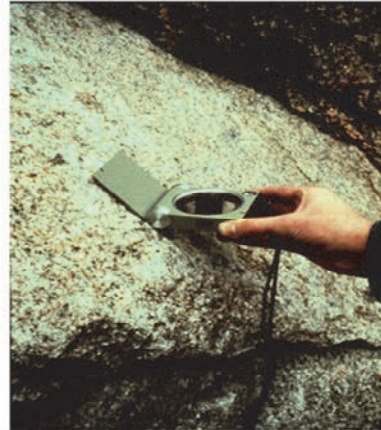
Measuring slope of joints using a structural compass
