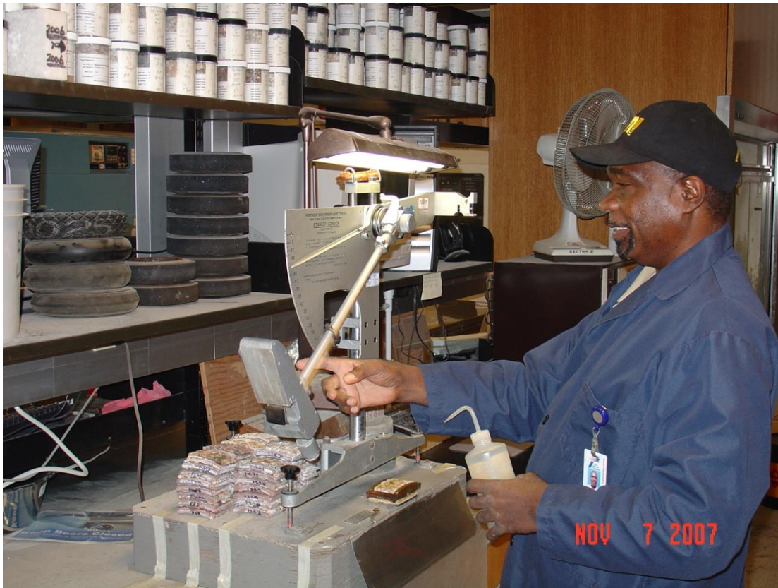
Figure 19: British Pendulum Tester in Use
