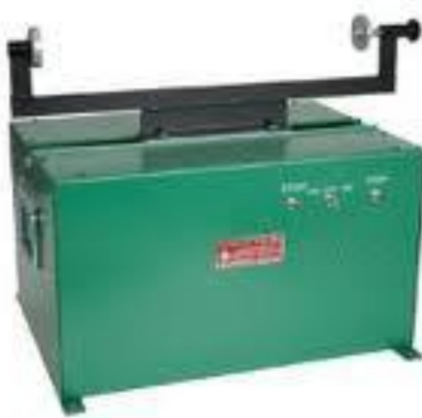
Figure 10: A typical mechanical shaker used to thoroughly disperse the sample in the cylinder
