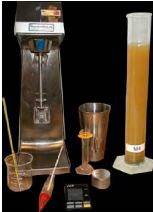
Figure 6: Equipment most frequently used in the T 88 procedure
