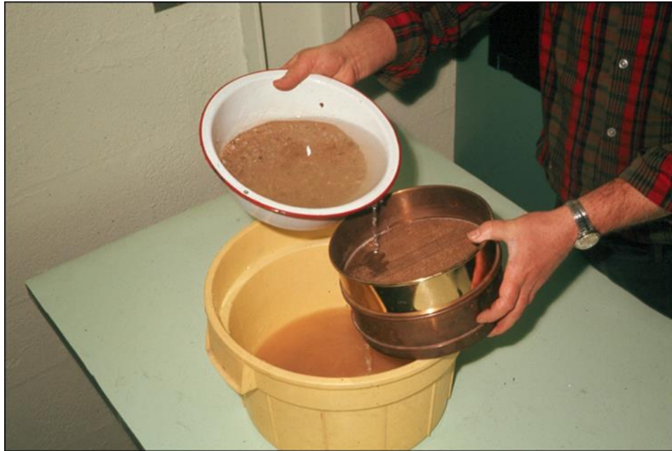
Figure 5: Final stages of washing over the #200 sieve for a fine aggregate sample
