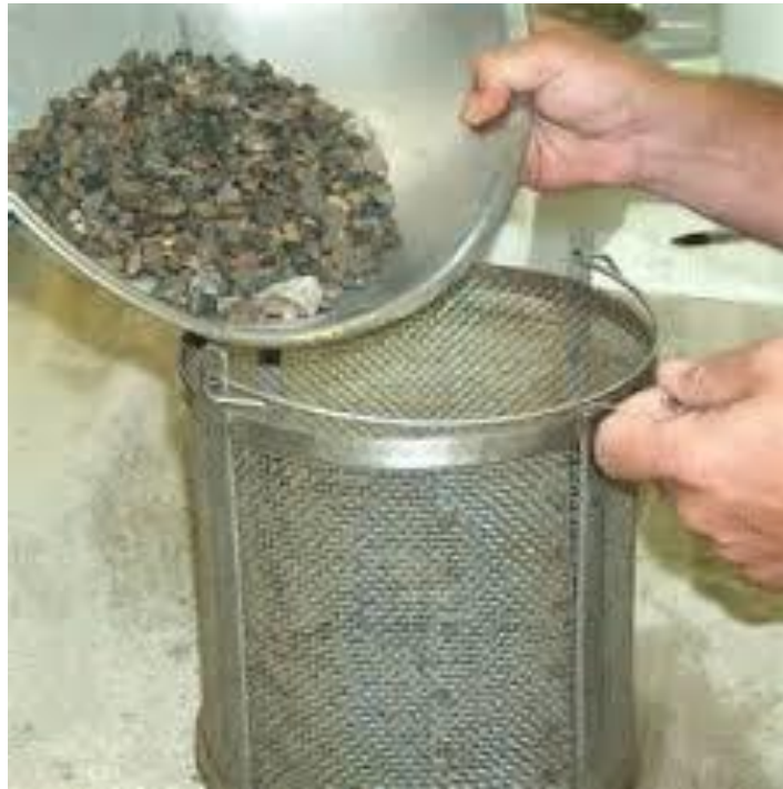
Figure 34: Prepared sample being placed in the weighing basket
