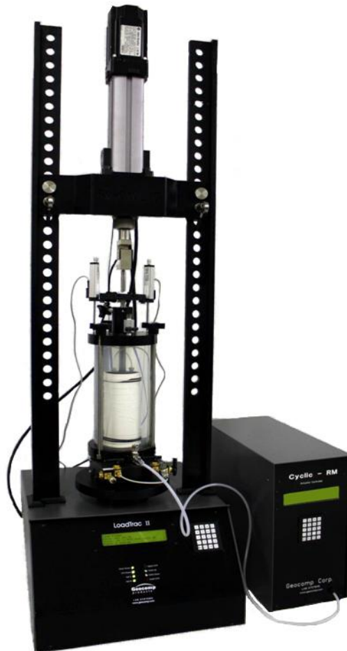
Figure 14: Load frame, linear actuator, triaxial cell with sample in place and the data acquisition system
