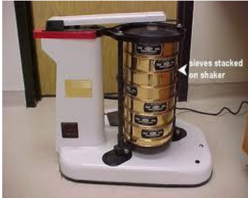
Figure 2: Sieve stack in the shaker
