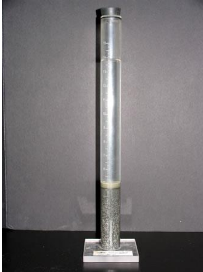
Figure 8: Graduated cylinder with sample already shaken and settled
