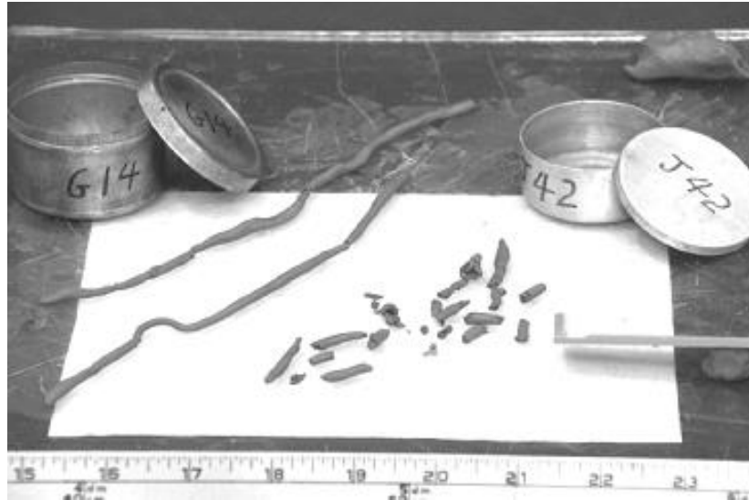
Figure 13: Plastic limit of the minus # 40 size fraction
