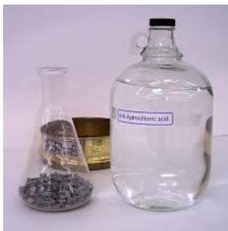
Figure 20: Incidental equipment used in ASTM D 3042
