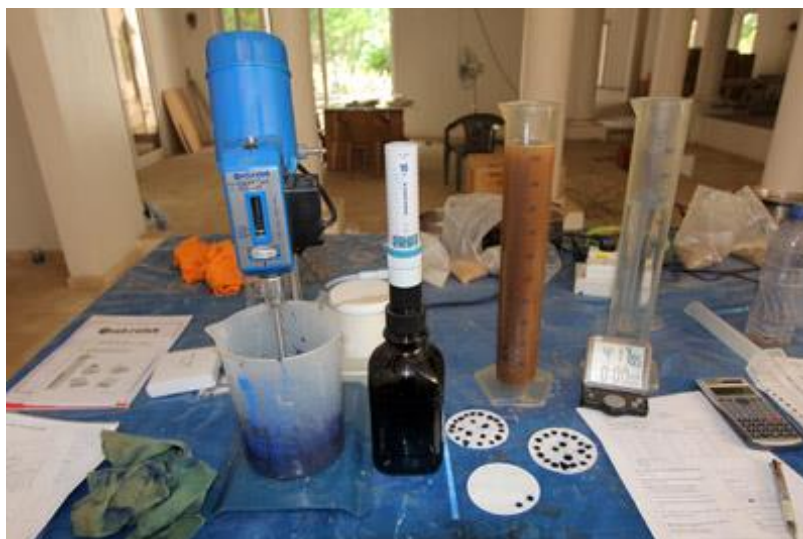
Figure 11: Equipment required to perform the methylene blue test
