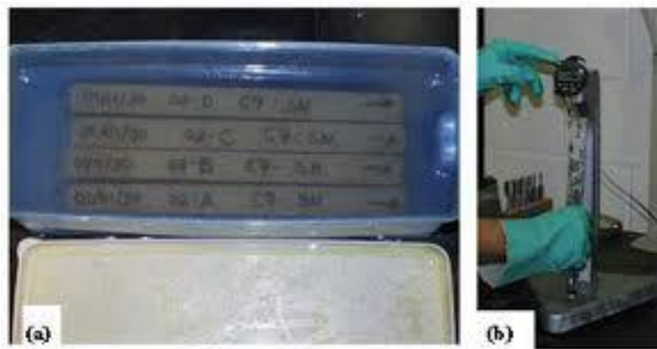
Figure 38: This figure includes two photos of 1260 testing. The first photo shows the mortar specimens placed submerged in NaOH solution within a blue storage container. The second photo shows a mortar bar specimen's length being measured.
