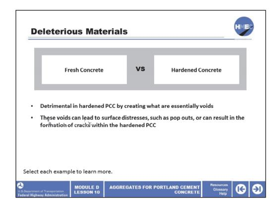
Deleterious materials effect both fresh and hardened PCC properties and can encompass many types of contamination, ranging from soft and friable aggregate particles to vegetable matter that may have been introduced during hauling or storage.
