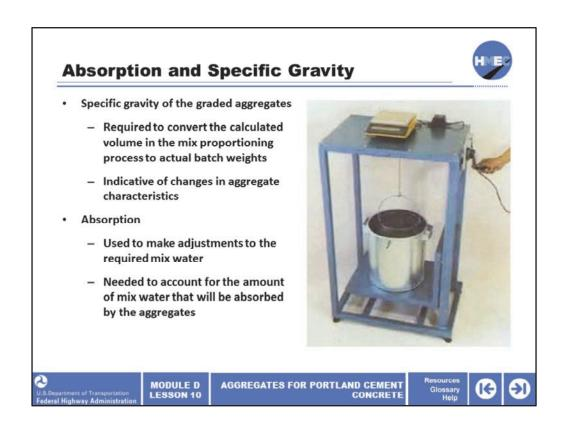
The absorption and specific gravity of coarse aggregates, as determined by AASHTO T 85, are important aggregate properties for fresh PCC.
