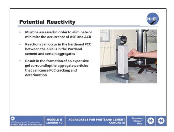
Reactivity is determined by numerous ASTM specifications that range in duration from several weeks to over a year. In this case, reactivity refers to the potential for an adverse reaction to occur between alkalis in the Portland cement and certain compounds within the aggregates.
