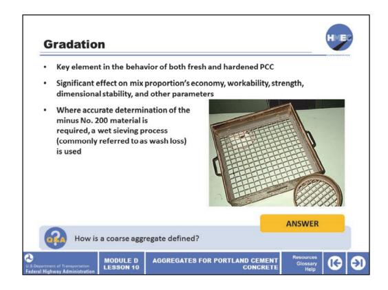
Gradation, as determined by a sieve analysis (AASHTO T 27), is one of the most important aggregate parameters for both fresh and hardened PCC. The gradation establishes the maximum and nominal maximum aggregate sizes as well as the size distribution of particles. The PCC mix design and proportioning procedure is dependent on these parameters.
