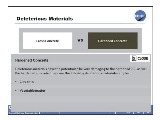
Deleterious materials have the potential to be very damaging to the hardened PCC as well. In the case of clay balls, these particles will disintegrate in service and result in surface distresses (pop outs) or the creation of voids in the PCC. Vegetable matter will similarly deteriorate over time and result in a void in the PCC, which reduces strength and durability.
