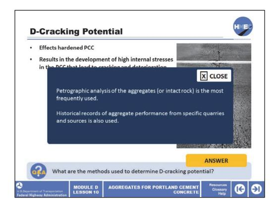
Petrographic analysis of the aggregates (or intact rock) is the most frequently used method to determine D-cracking potential. Historical records detailing aggregate performance from specific quarries and sources is also used.
