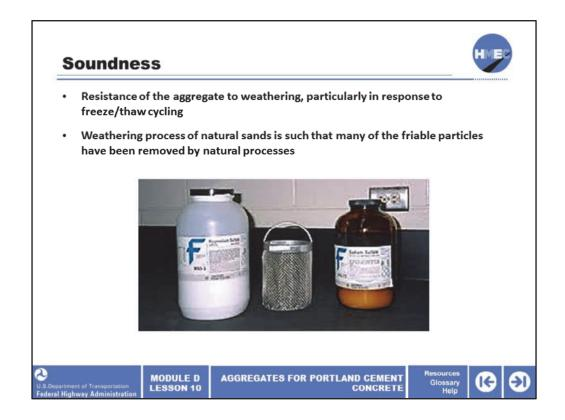
The soundness of aggregates is an important fine aggregate characteristic in hardened PCC, and is equally important in fine and coarse aggregates.
