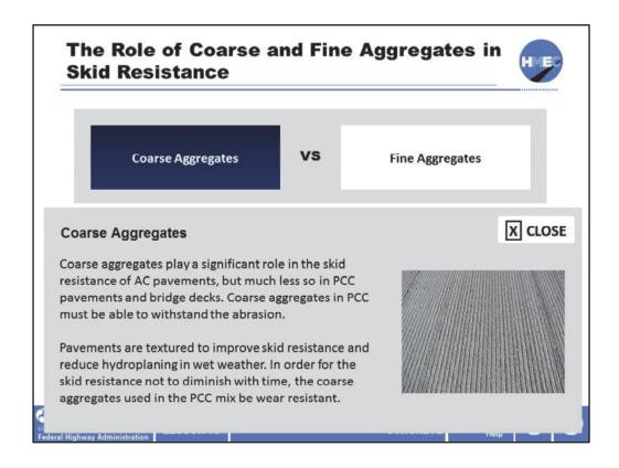
Coarse aggregates play a significant role in the skid resistance of AC pavements, but much less so in PCC pavements and bridge decks.
