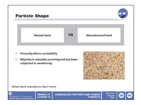
The particle shape of the fine aggregate primarily influences the properties of fresh PCC. Generally, the most effected property is workability as it is a function of gradation, particle shape, and surface texture of the aggregates.
