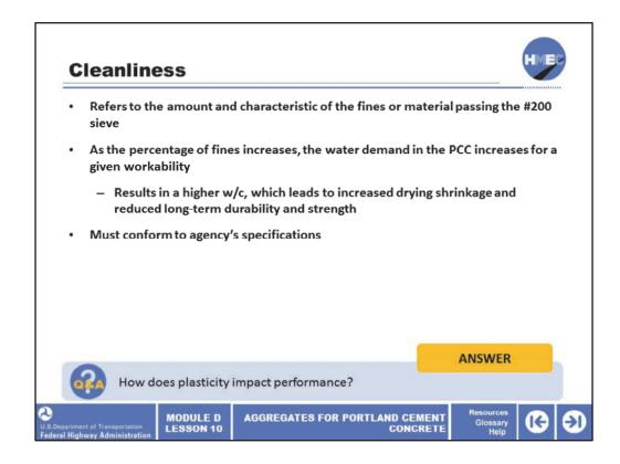
The cleanliness of the fine aggregates is an important property in fresh PCC, as it was for coarse particles. Although the immediate effects are in the fresh PCC, there are long-term effects on the hardened PCC.
