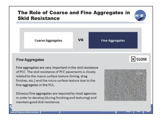
Fine aggregates are very important in the skid resistance of PCC. The skid resistance of PCC pavements is closely related to the macro surface texture (tining, drag finishes, etc.) and the micro surface texture due to the fine aggregates in the PCC.
