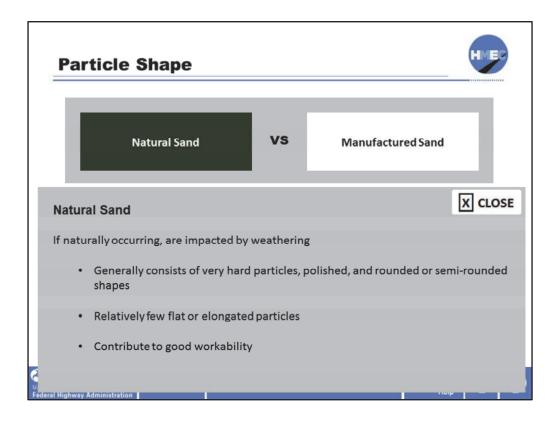
Natural sand that has been exposed to weathering generally consists of very hard particles, polished, and rounded or semi-rounded shapes. As a rule, there are relatively few flat or elongated particles. These shapes and smooth surface texture contribute to good workability and finishability in a correctly proportioned mix.
