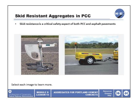
Skid resistance is a critical safety aspect of both PCC and asphalt pavements. Skid resistance is based on the friction that is developed between the pavement surface and tires. The skid resistance of the roadway is well correlated to accident rates, particularly on curves, at intersections and during wet weather.
