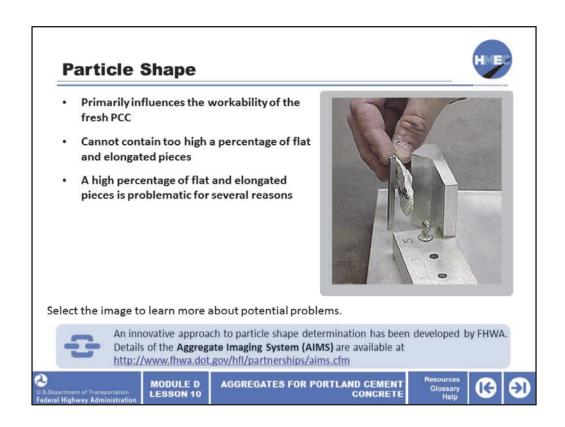
The particle shape of the coarse aggregate, as determined by ASTM D4791, primarily influences the workability of the fresh PCC, as flat and elongated particles do not readily reorient during placement and consolidation. Workability is a function of numerous variables, including the particle shape, which relates to the orientation and interaction between the aggregate particles during placement.
