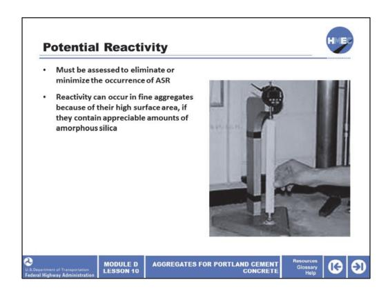
The potential reactivity of aggregates must be assessed in order to eliminate or minimize the occurrence of ASR. These reactions can occur in the hardened PCC between the alkalis in the Portland cement and certain aggregates containing amorphous or reactive silica.
