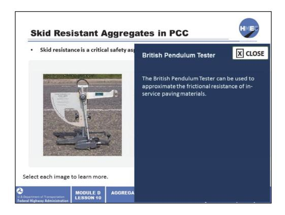
The British Pendulum Tester can be used to approximate the frictional resistance of inservice paving materials.
