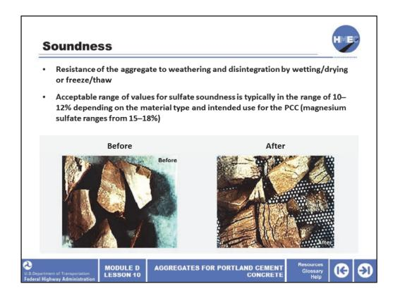
The soundness of coarse aggregates, as determined by the sodium or magnesium sulfate soundness test described in AASHTO T 104, is important for hardened PCC and is directly related to freeze/thaw durability (as is entrained air in the paste).
