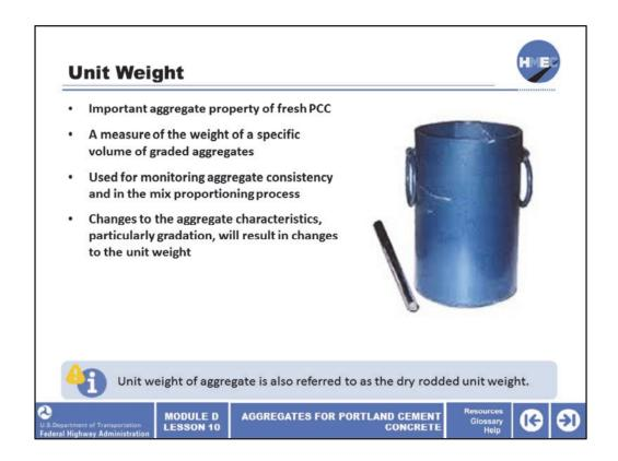
The unit weight of aggregates, as determined by AASHTO T 19, is an important aggregate property for fresh PCC. The unit weight (or dry rodded unit weight) is a measure of the weight of a specific volume of graded aggregates and is used for monitoring aggregate consistency and in the mix proportioning process.
