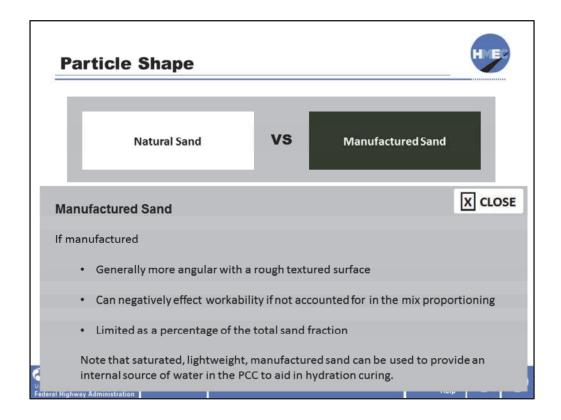
Manufactured sand is generally more angular with a rough textured surface that can negatively effect workability if not accounted for in the mix proportioning. Due to the nature of these particles, manufactured sand is generally limited as a percentage of the total sand fraction.
