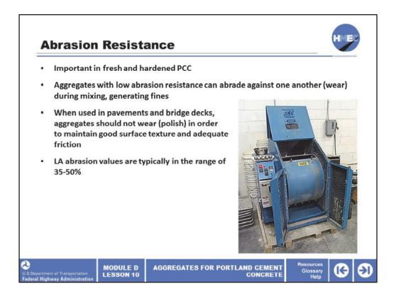
The abrasion resistance of the coarse aggregates, as determined according to AASHTO T 96 or T 327, is important in both fresh and hardened PCC. Abrasion resistance is important during the mixing process and also for the in-place PCC used in pavements and bridge decks.
