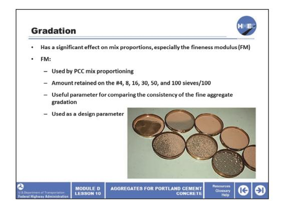
Fine aggregates impact the behavior of both fresh and hardened PCC properties. The gradation of fine aggregates, which is determined by a sieve analysis (AASHTO T 27), has a significant effect on mix proportions, particularly the fineness modulus (FM).
