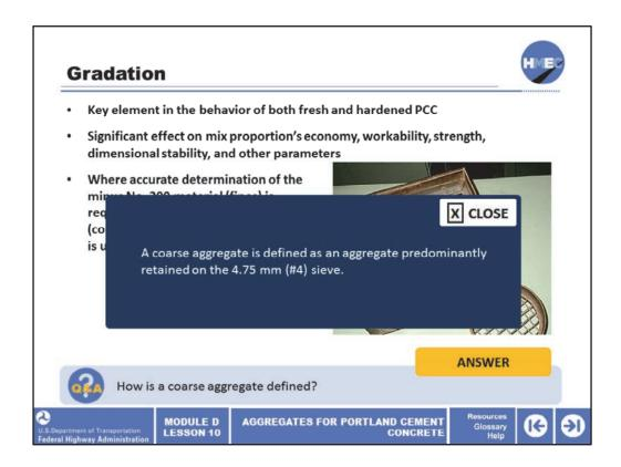
A coarse aggregate is defined as an aggregate predominantly retained on the 4.75 mm (#4) sieve.
