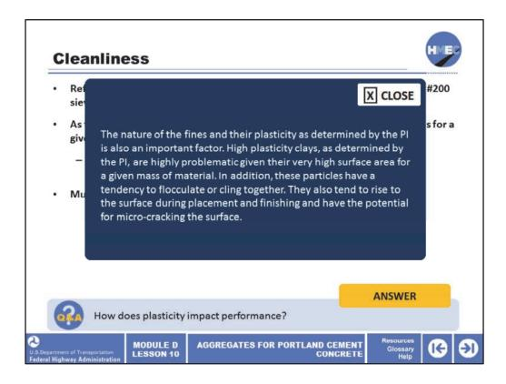
The nature of the fines and their plasticity as determined by the PI is also an important factor. High plasticity clays, as determined by the PI, are highly problematic given their very high surface area for a given mass of material. In addition, these particles have a tendency to flocculate or cling together. They also tend to rise to the surface during placement and finishing and have the potential for micro-cracking the surface.
