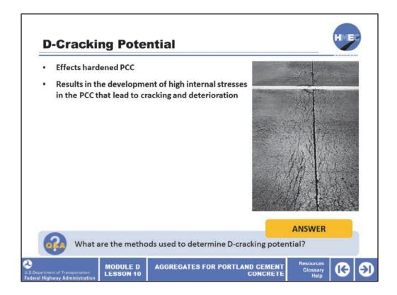
D-cracking is basically the expansion of susceptible coarse aggregate particles due to water freezing in the aggregate voids. The expansion results in the development of high internal stresses, which leads to cracking of the PCC.
