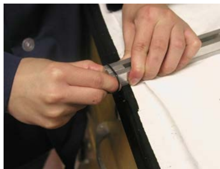
Figure 40: Placing O-ring on the end of the mold
