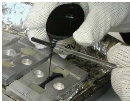
Figure 49: Pouring asphalt binder into heated molds
