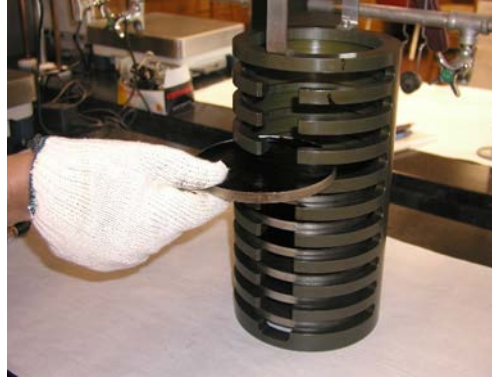
Figure 31: Placing sample pans in the holder
