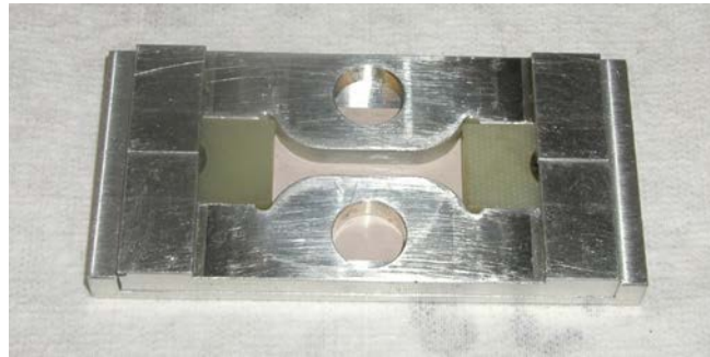
Figure 47: Side plates inserted into mold
