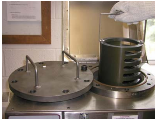
Figure 29: Placing sample holder in the chamber
