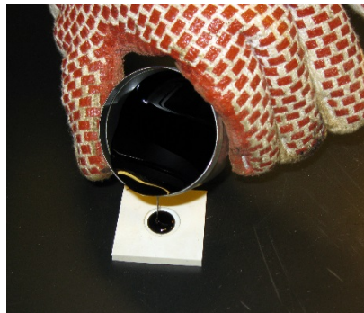
Figure 8: Pouring asphalt in silicone mold
