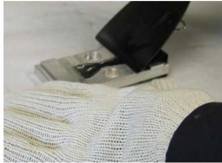
Figure 50: Trimming the test specimens
