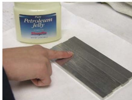
Figure 37: Applying petroleum grease to molds
