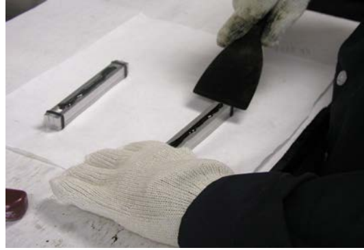
Figure 42: Trimming test specimens
