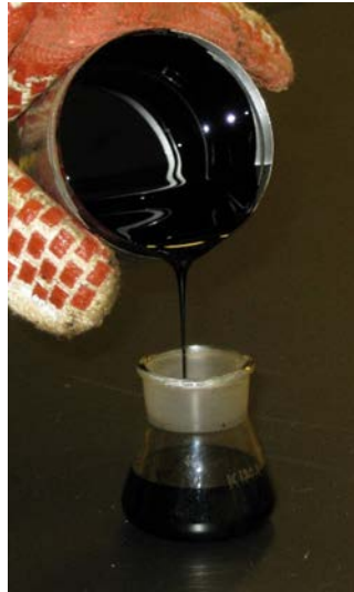
Figure 3 – Pouring asphalt binder into pycnometer
