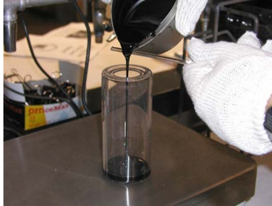
Figure 21: Pouring 35 \pm 0.5 g of binder into each container
