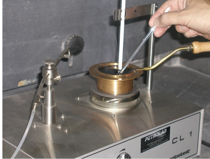
Figure 12: Removing skin from sample surface
