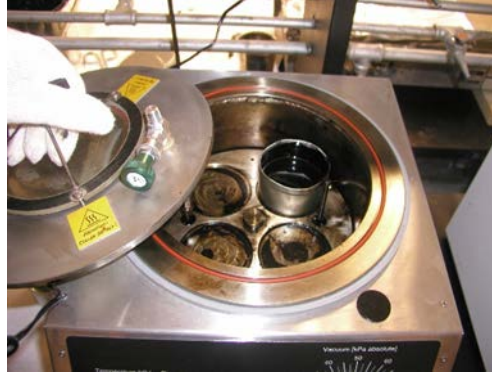
Figure 35: Placing the sample in the degassing oven
