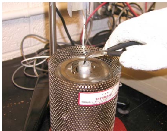
Figure 15: Inserting the sample chamber into the thermosel
