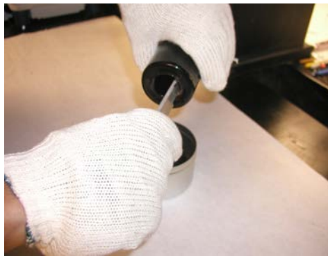
Figure 25: Scraping material from the wall of the container
