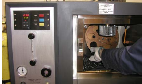
Figure 23: Placing samples in rotating carriage
