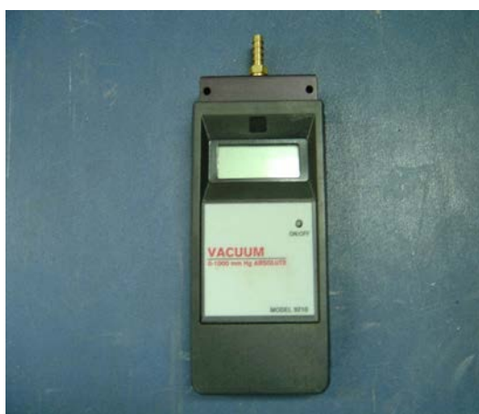
Figure 7: Digital pressure gauge
