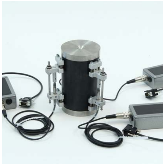
Figure 11: LVDTs Mounted to a Dummy Specimen in a 120° Configuration
