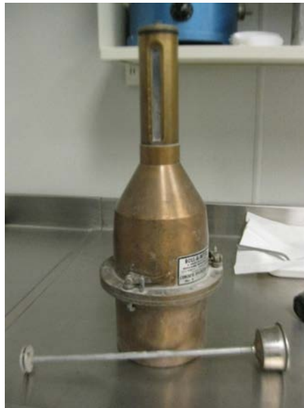
Figure 2: A typical brass volumetric meter
