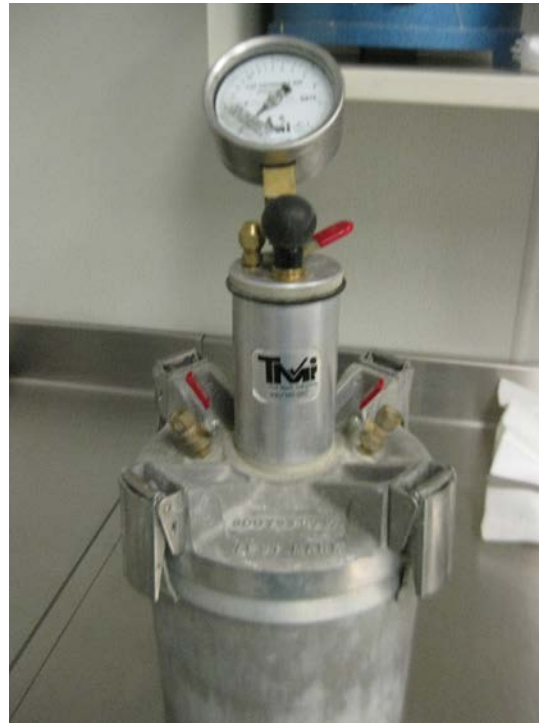
Figure 1: Type B air meter
