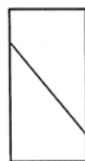
Type 4 Diagonal fracture with no cracking through ends; tap with hammer to distinguish from Type 1
