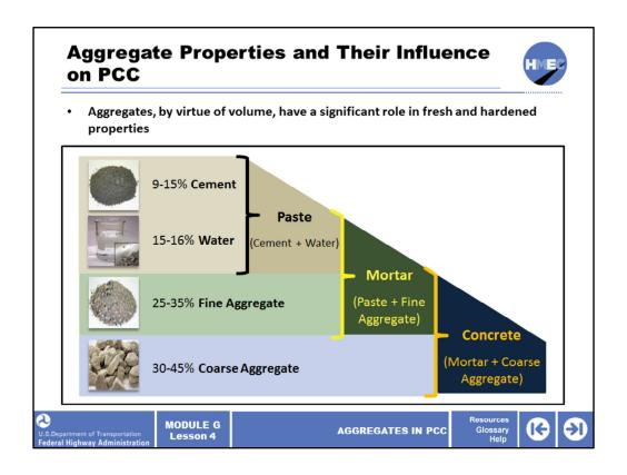
Aggregates, by virtue of their volume, have a significant role in both fresh and hardened properties of a PCC mix.
