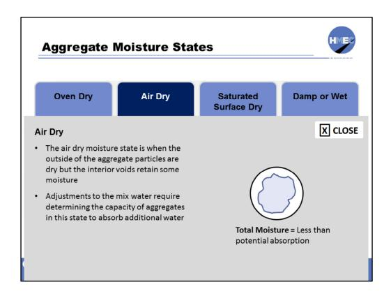
The air dry moisture state is when the outside of the aggregate particles are dry but the interior voids retain some moisture. Adjustments to the mix water require determining the capacity of aggregates in this state to absorb additional water.
