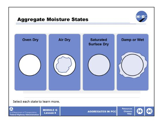
There are four moisture states of aggregates: oven dry, air dry, saturated surface dry, and damp or wet. Select each state to learn more.
