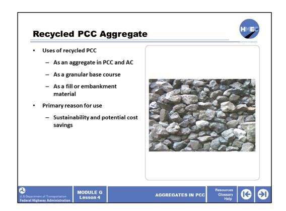
Recycled PCC is frequently used in both rigid and flexible pavement construction. The most common uses include an aggregate in PCC or asphalt concrete (AC) mixes, a base or subbase material, and as an embankment or fill material.
