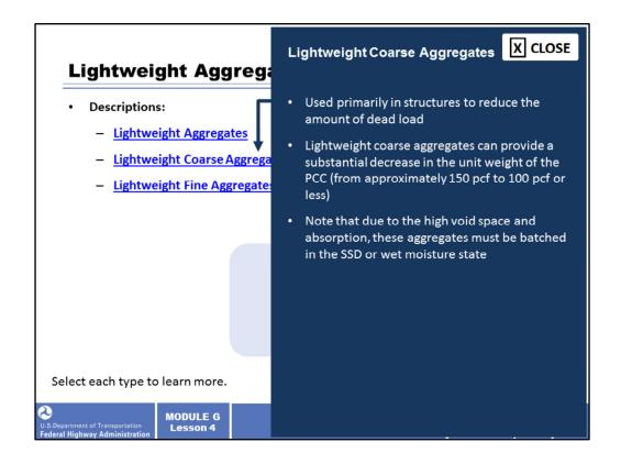
Lightweight coarse aggregates are used primarily in structures to reduce the amount of dead load.
