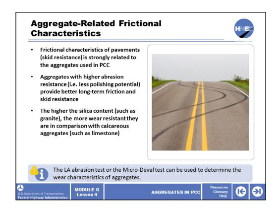
The frictional characteristics of pavements (skid resistance) is strongly related to the aggregates used in PCC. Although there is not a definitive relationship established, higher abrasion resistance results in improved long-term friction and better skid resistance.
