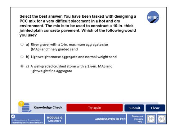
Select the best answer. You have been tasked with designing a PCC mix for a very difficult placement in a hot and dry environment. The mix is to be used to construct a 10 in. thick jointed plain concrete pavement. Which of the following would you use?
