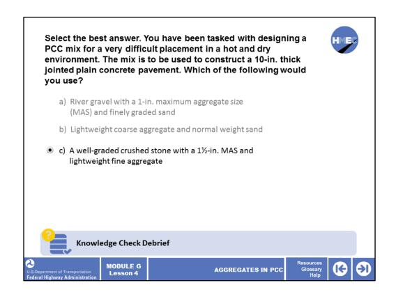
The correct answer is c) A well-graded crushed stone with a 1½-in. MAS and lightweight fine aggregate.
