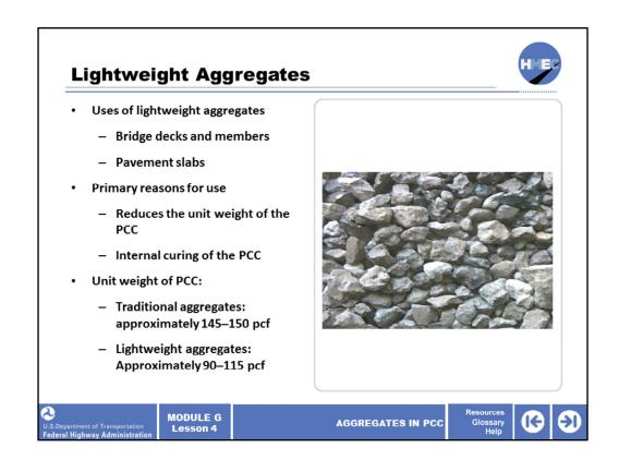
Lightweight aggregates are used in a variety of applications, including bridge decks and members and pavement slabs. The primary reason for using lightweight coarse aggregate is to reduce the unit weight of the PCC, thereby reducing the size of the structural elements due to dead loads. Normal weight PCC is approximately 145–150 pounds per cubic foot (pcf) compared to lightweight PCC at 90–115 pcf.
