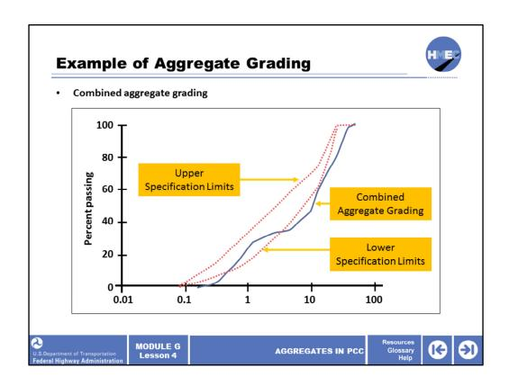
This example shows a combined aggregate grading, which is represented by the blue line. The upper and lower specification limits for this aggregate are shown by the two red dashed lines. Note that the gradation shown falls outside of the specifications on the lower bound.
