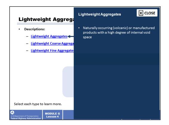
Lightweight aggregates are naturally occurring (volcanic) or manufactured products with a high degree of internal void space.
