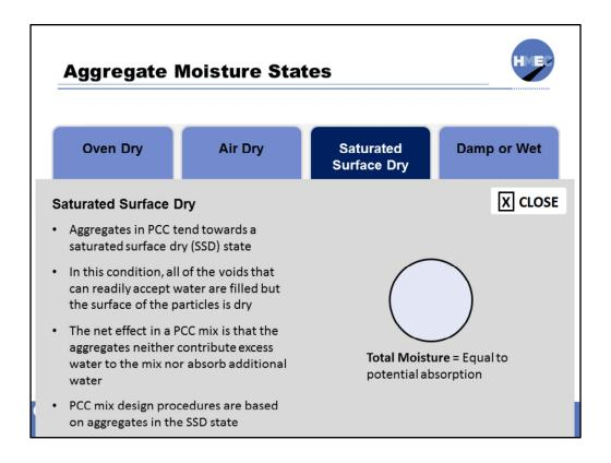
Aggregates in PCC tend towards a saturated surface dry (SSD) state. In this condition, all of the voids that can readily accept water are filled but the surface of the particles is dry. The net effect in a PCC mix is that the aggregates neither contribute excess water to the mix nor absorb additional water. PCC mix design procedures are based on aggregates in the SSD state.
