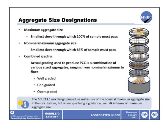
The maximum aggregate size and nominal maximum size are important from a mix design standpoint as well as in the performance of the fresh and hardened PCC.
