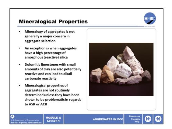
The mineralogy of the aggregates is not generally a major concern in aggregate selection. An exception to this is when the aggregates have a high percentage of amorphous (reactive) silica, which can lead to alkali-silica reactivity. In addition, dolomitic limestones with small amounts of clay are also potentially reactive and can lead to alkali-carbonate reactivity.
