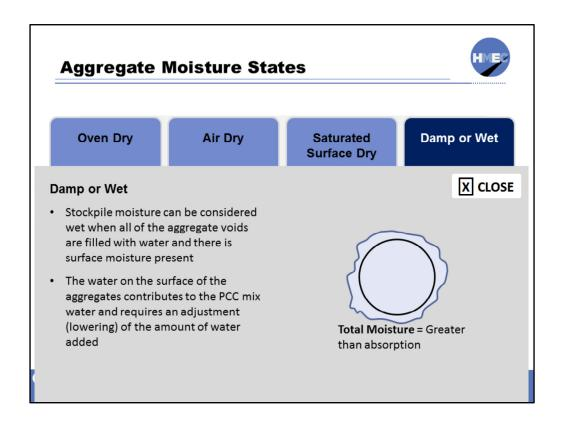
Stockpile moisture can be wet, in which case the water on the surface of the aggregates contributes to the PCC mix water. If no adjustments were made to the mix proportions, the surface water would raise the w/c ratio. Note that this moisture state generally exists after periods of sustained rainfall (unprotected stockpiles) or when stockpiles are misted to reduce temperature or equilibrate moisture.
