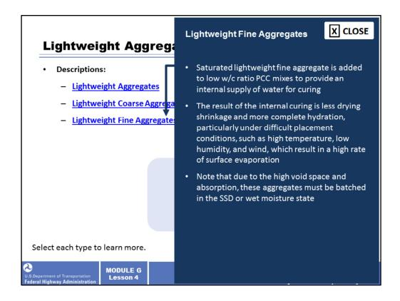
Lightweight fine aggregates are sometimes used to provide internal curing by providing moisture within low w/c ratio PCC during hydration.
