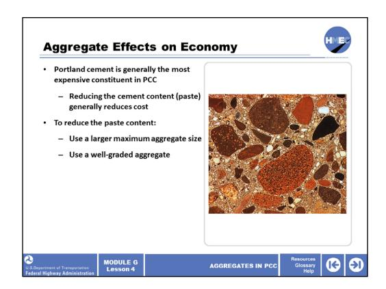
Portland cement is generally the most expensive constituent in PCC, therefore, reducing the cement content (paste) generally reduces cost. To reduce the paste content, you can do the following:
