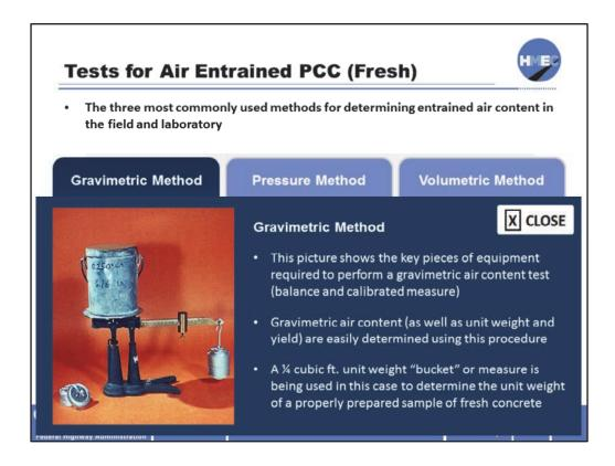
This picture shows the key pieces of equipment required to perform a gravimetric air content test (balance and calibrated measure). Gravimetric air content (as well as unit weight and yield) are easily determined using this procedure. The mix proportions and properties must be known in order to use this method for air void determination. A ¼ cubic ft. unit weight "bucket" or measure is being used in this case to determine the unit weight of a properly prepared sample of fresh concrete.
