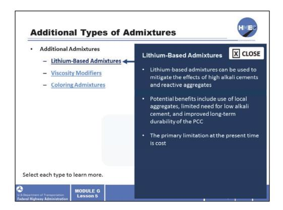
Lithium-based admixtures can be used to mitigate the effects of high alkali cements and reactive aggregates. Potential benefits include use of local aggregates, limited need for low alkali cement, and improved long-term durability of the PCC. The primary limitation at the present time is cost.
