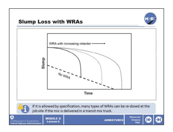
The slump loss behavior of various types of WRAs are shown in this figure. The chemistry of the overall system (cement, water, other admixtures) and temperature play a key role in this behavior. The best way to gauge slump loss with a particular mix (with other admixtures) is to perform trial batches under the most likely placement conditions. Note that if it is allowed by specification, many types of WRAs can be re-dosed at the job site if the mix is delivered in a transit mix truck.
