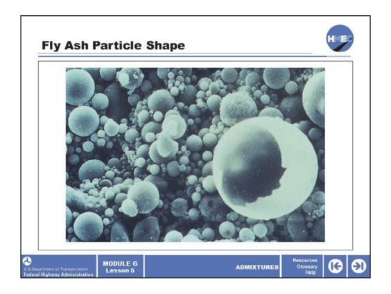
This scanning electron microscope photo shows the spherical nature of fly ash. Note the glassy and smooth surface texture that can result in a decreased water demand when a portion of the cement is replaced with fly ash. Note the wide variation in particle size. The addition of fly ash improves workability due to the lubricating action of the spherical particles.
