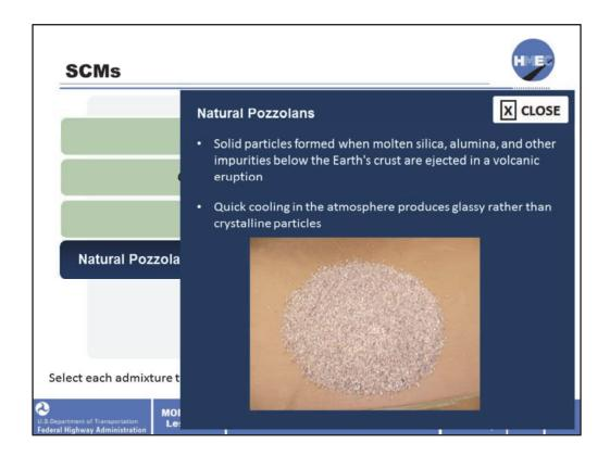
Natural pozzolans are solid particles formed when molten silica, alumina, and other impurities below the Earth's crust are ejected in a volcanic eruption. Quick cooling in the atmosphere produces glassy rather than crystalline particles.
