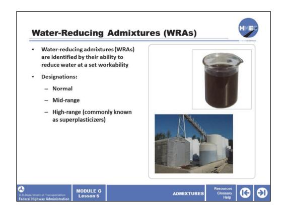
Water-reducing admixtures (WRAs) are identified by their ability to reduce water at a set workability. The three designations listed perform the same basic function of allowing the use of a reduced amount of water while maintaining workability. They are:
