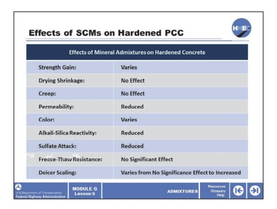
As stated in the preceding slide, the degree to which each of these properties are affected is governed by the specific properties of the SCMs admixture, characteristics of the PCC mix, and environmental conditions.
