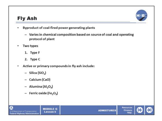
Fly ash is a byproduct of coal-fired power generating plants and varies in chemical composition based on the source of coal and the operating protocol of the plant. Fly ash is considered a waste product and the chemical composition can vary on a routine basis. There are two types of fly ash: Type F and Type C. The two types are comprised of essentially the same compounds only in different quantities. The active or primary compounds in fly ash include:
