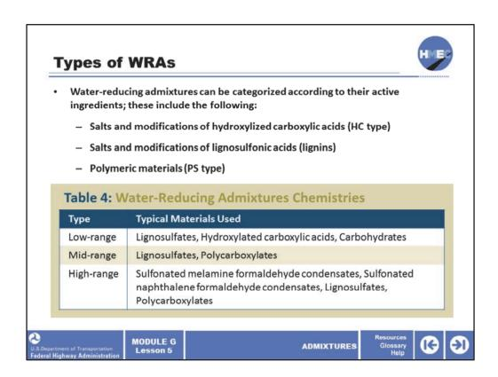
There are three basic families of WRAs as shown on this slide. The effectiveness of the WRA is dependent on the chemistry of the admixture and the dose. Each of the materials shown has specific properties but are somewhat variable based on the manufacturers formulation.
