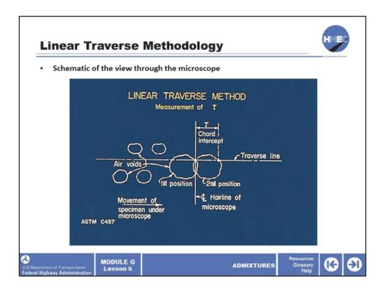
Here we see a schematic of the view through the microscope, illustrating the voids, traverse line, and direction of movement. As can be seen, the measurements must be very precise in order to produce representative results.
