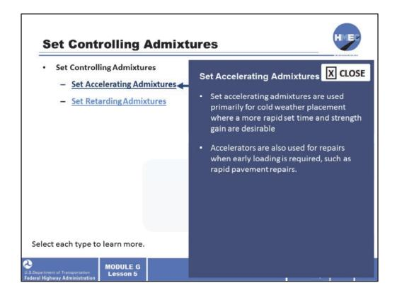
Set accelerating admixtures are used primarily for cold weather placement where a more rapid set time and strength gain are desirable.
