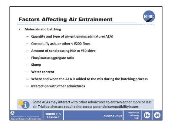
The required air content is related to the environmental exposure conditions of the PCC, the combined aggregate gradation, the cement content, the total water content, and other factors that will be discussed in the mix proportioning lesson. The entrained air content of a PCC mix is accounted for in the initial mix proportioning calculations.
