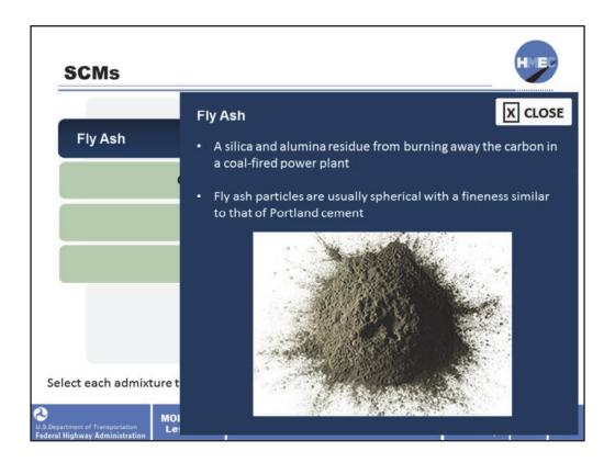
Fly ash is a silica and alumina residue from burning away the carbon in a coal-fired power plant. Fly ash particles are usually spherical with a fineness similar to that of Portland cement.
