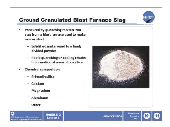
The use of ground granulated blast furnace slag is growing steadily due to its relatively low cost and the beneficial properties it imparts to a PCC mix. GGBFS is another of the industrial byproducts that has found application in PCC production. GGBFS is produced by quenching molten iron slag from a blast furnace used to make iron and steel.
