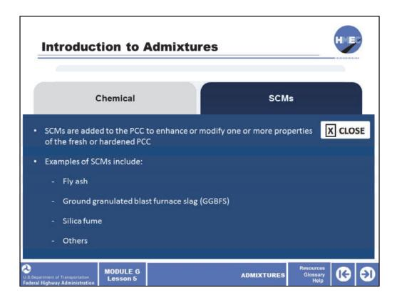
Examples of SCMs include fly ash, ground granulated blast furnace slag, silica fume, and others.
