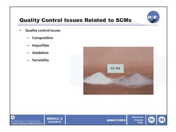
Due to the majority of SCMs being industrial byproducts (particularly fly ash), quality control issues may arise in their use. The exception being when these materials are processed specifically for use in PCC and therefore have tight controls. SCMs quality control issues generally fall into one or more of the following four categories:
