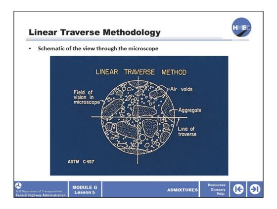
The image depicts the schematic field of view looking through the microscope. Note the line of traverse and the number, variation in size, and spacing between the air voids on the line of traverse. Statistical methods are used to estimate the air void parameters in three dimensions based on these values.
