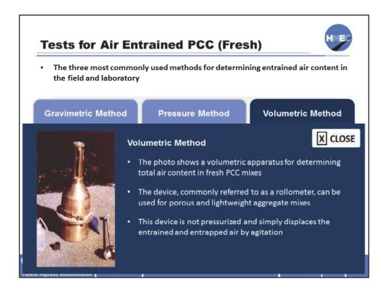
The photo shows a volumetric apparatus for determining total air content in fresh PCC mixes. The device, commonly referred to as a rollometer, can be used for porous and lightweight aggregate mixes. This device is not pressurized and simply displaces the entrained and entrapped air by agitation.
