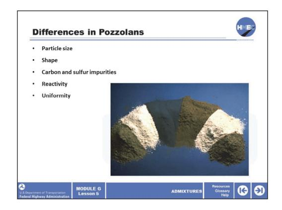
Although SCMs are fundamentally the same, there are important differences, including size, shape, carbon and sulfur impurities, and reactivity. (Not all silica is converted to glass in any process. Some portion is crystalline and therefore less reactive.) The day-to-day uniformity of the product also depends on the day-to-day uniformity of the process.
