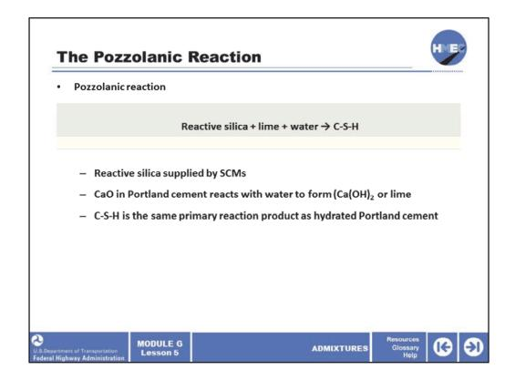
The pozzolanic reaction is a very important attribute of these four types of SCMs. They do not simply act as a finely divided filler, they actually produce cementing products. Here is an example of a pozzolanic reaction:
