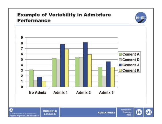
The graph here, shows the air content of a PCC mix using the same mix proportions. Note the differences in air content with no admixtures present and the relative differences due to the addition of three admixtures. The differences are due to the physical and chemical properties of the cements and the chemical properties of the admixtures.
