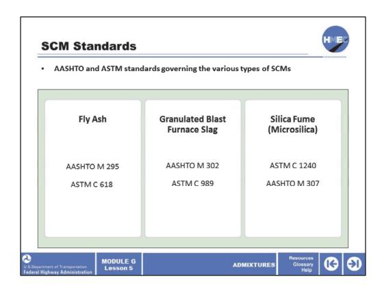
Both AASHTO and ASTM have standards governing the various types of SCMs. As previously mentioned, SCMs are generally an industrial byproduct that can be processed or unprocessed depending on the material. The standards are specific in terms of physical properties and limitations on compounds that can be detrimental to the performance of PCC. Here are some references for various types of SCMs.
