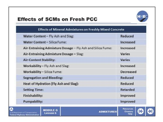
The degree to which each of these properties are affected is governed by the specific properties of the SCMs admixture, characteristics of the PCC mix, and environmental conditions.
