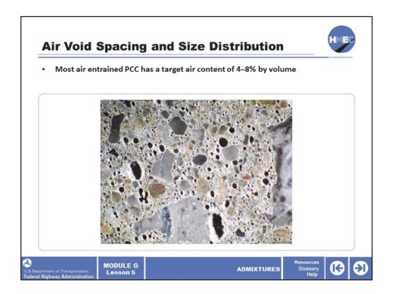
Most air entrained PCC has a target air content of 4–8% by volume. Entrapped air voids are not a desirable characteristic due to their size and random spacing. These types of voids do not provide freeze/thaw resistance and reduce PCC strength. Entrained air consists of millions of very small voids uniformly distributed throughout the cement paste.
