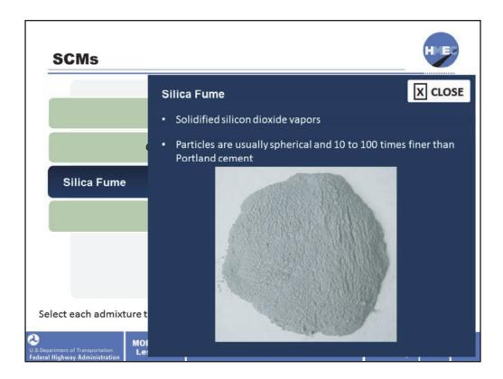
Silica fume is solidified silicon dioxide vapors. Particles are usually spherical and 10 to 100 times finer than Portland cement.
