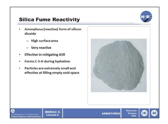
Silica fume is an amorphous (reactive) form of silicon dioxide and due to its extremely high surface area is very reactive. As with fly ash, silica fume has been shown to be effective in mitigating ASR. This material forms C-S-H during hydration, as was previously discussed in regards to the pozzolanic reaction. Silica fume particles are extremely small and are very effective at filling the empty void space between the cement grains.
