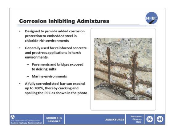
Corrosion inhibiting admixtures are designed to provide added corrosion protection to embedded steel in chloride rich environments. These admixtures are generally used for reinforced concrete and prestress applications in harsh environments. Chloride-rich environments include pavements and bridges exposed to deicing salts as well as marine environments.
