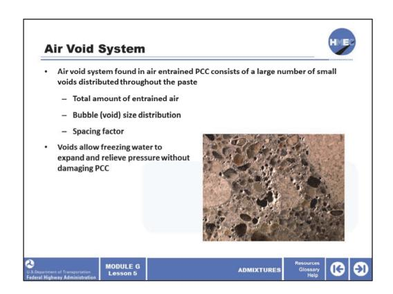
The air void system found in air entrained PCC consists of a large number of very small voids distributed throughout the paste. The air void system is based on the total amount of entrained air, the bubble (void) size distribution, and the spacing factor. The air-entraining admixture is used to create stable microscopic bubbles that result in voids in the hardened PCC.
