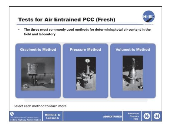
There are a number of methods to determine the volume of air voids in fresh PCC. The three most commonly used methods for determining total air content in the field and laboratory are:
