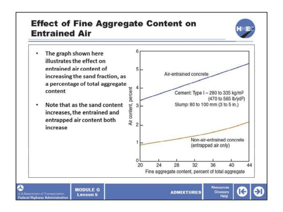
The graph shown here illustrates the effect on entrained air content of increasing the sand fraction, as a percentage of total aggregate content. Note that as the sand content increases, the entrained and entrapped air content both increase. This difference is not due strictly to the increased sand content, but on changes to the other mix proportions to compensate for the varying sand/coarse aggregate ratio (changed cement and water content).
