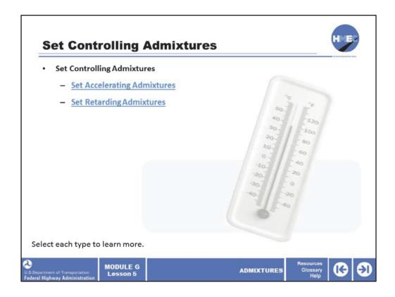
Set controlling admixtures are generally used for hot and cold weather PCC placement. They are widely used to control the set time and rate of strength gain under adverse placement conditions. They are also used for long haul distances and times. Some different types of set controlled admixtures are:
