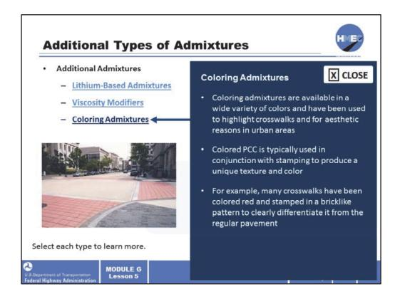
Coloring admixtures are available in a wide variety of colors and have been used to highlight crosswalks and for aesthetic reasons in urban areas. Colored PCC is typically used in conjunction with stamping to produce a unique texture and color. For example, many crosswalks have been colored red and stamped in a bricklike pattern to clearly differentiate them from the regular pavement.
