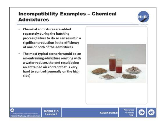
Chemical admixtures are added separately during the batching process. Failure to do so can result in a significant reduction in the efficiency of one or both of the admixtures. The most typical scenario would be an air-entraining admixture reacting with a water reducer, the end result being an entrained air content that is very hard to control (generally on the high side).
