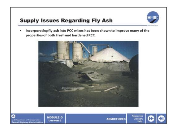
Incorporating fly ash into PCC mixes has been shown to improve many of the properties of both fresh and hardened PCC. Fly ash has been readily available since most electrical power generation plants have traditionally been coal fired. While still readily available in most parts of the US, fly ash, by virtue of it being a byproduct of coal-fired power generation facilities, will likely become harder to obtain as energy policies move us away from the use of coal.
