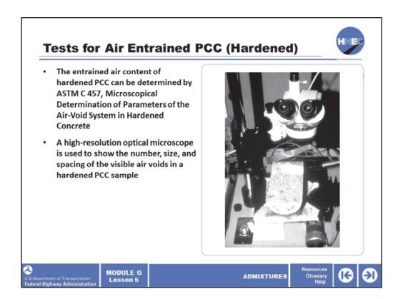
This test method, commonly referred to as the linear traverse method, requires specialized equipment and a specifically trained technician to perform correctly. A high-resolution optical microscope is used to show the number, size, and spacing of the visible air voids in a hardened PCC sample.
