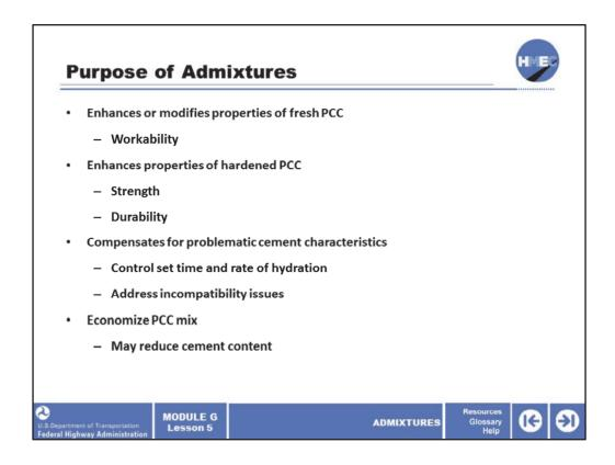
Admixtures are used for a variety of reasons, ranging from modifying the physical properties of the PCC to saving money. One of the primary uses of admixtures is to enhance the properties of fresh PCC. Equally important, admixtures are used to enhance one or more properties of hardened PCC, to compensate for potentially problematic cement characteristics and to economize the PCC mix.
