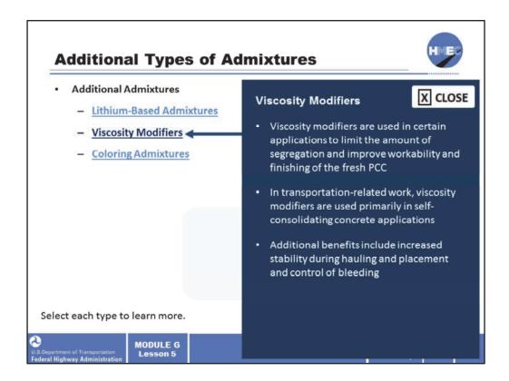
Viscosity modifiers are used in some applications to limit the amount of segregation and improve workability and finishing of the fresh PCC. In transportation-related work, viscosity modifiers are used primarily in self-consolidating concrete applications. Additional benefits include increased stability during hauling and placement and control of bleeding.
