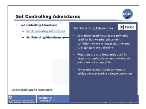
Set retarding admixtures are primarily used for hot weather placement conditions where a longer set time and strength gain are desirable.
