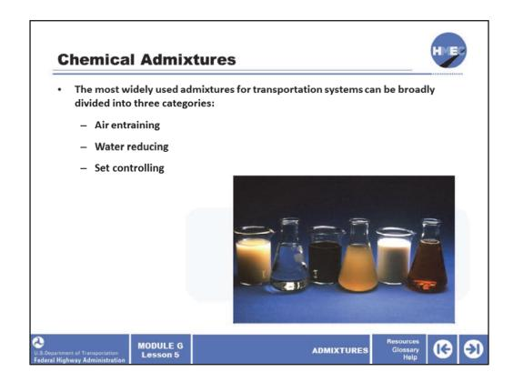
The most widely used admixtures for transportation systems can be broadly divided into three categories:
