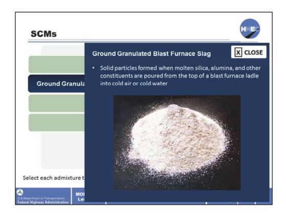
Ground granulated blast furnace slag are solid particles formed when molten silica, alumina, and other constituents are poured from the top of a blast furnace ladle into cold air or cold water.
