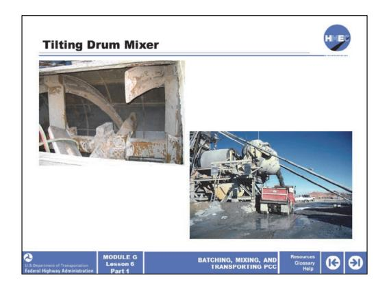
The blades or paddles and the mixing action of a central-mix drum are quite different than a truck mixer, where there is little folding action compared with that in a stationary mixer. The photo on the left illustrates the mixing blades inside a central-mix drum.
