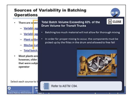
Batching too much material will not allow for thorough mixing. Refer to ASTM C94.
