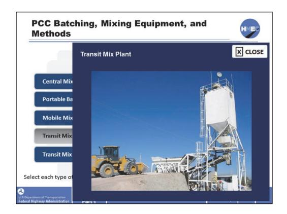
The photo shows a typical transit mix plant. Unlike the central mix plants, the production rate is not controlled as much by the plant as by the number of trucks and charging rate per truck. The end loader pictured feeds aggregates to the plant where they are batched into the transit mix trucks according to the mix proportioning. The silo stores both cement and SCMs and discharges into the trucks by gravity.
