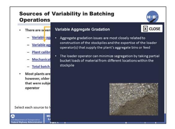
Aggregate gradation issues are most closely related to construction of the stockpiles and the expertise of the loader operator(s) that supply the plant's aggregate bins or feed.
