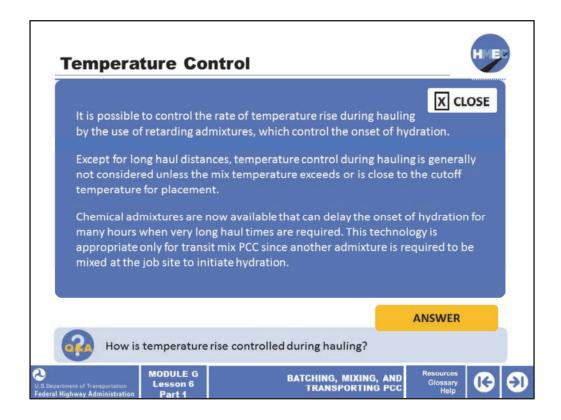
It is possible to control the rate of temperature rise during hauling by the use of retarding admixtures, which control the onset of hydration.
