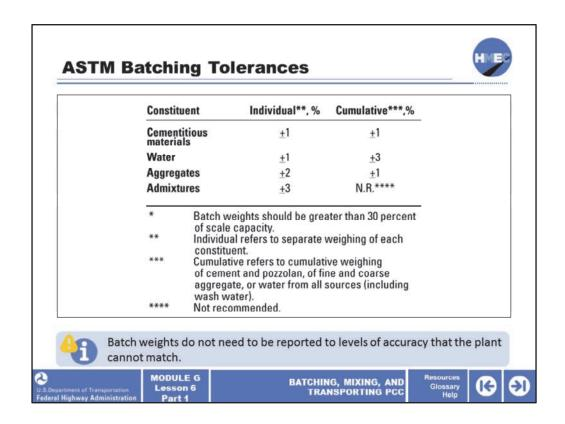
The batching tolerances established by ASTM govern all of the primary PCC components.
