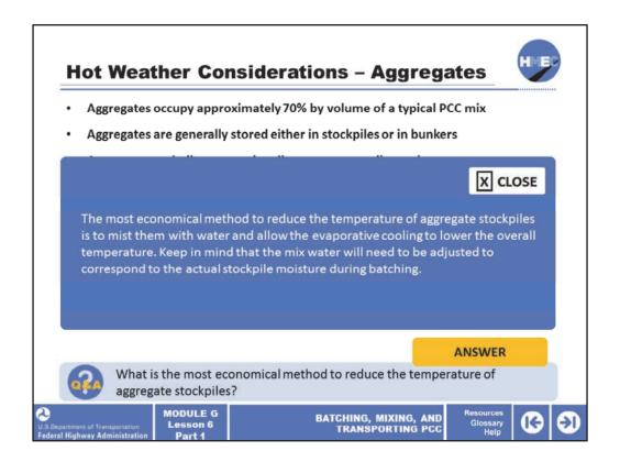
The most economical method to reduce the temperature of aggregate stockpiles is to mist them with water and allow the evaporative cooling to lower the overall temperature. Keep in mind that the mix water will need to be adjusted to correspond to the actual stockpile moisture during batching.
