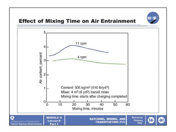
In order for the entrained air bubbles to develop in PCC, air has to be introduced into the PCC through mixing. The stability of the bubbles is then controlled by the air entraining admixture.
