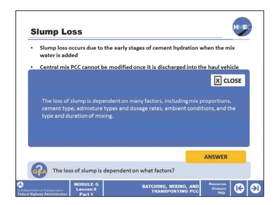
The loss of slump is dependent on many factors, including mix proportions, cement type, admixture types and dosage rates, ambient conditions, and the type and duration of mixing.
