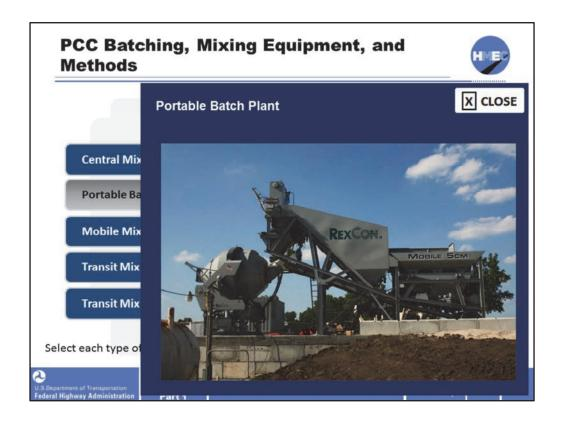
The photo shows a smaller portable batch plant. The production rate of this plant is approximately 130 cy per hour but is much more easily transported and erected at the job site than the plant on the previous slide.
