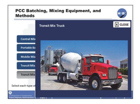
The photo shows a rear discharge transit mix truck. The mixing drum is visible as is the plant in the background. There are numerous variations in the configurations of these trucks, including front and rear discharge and a range of drum sizes.
