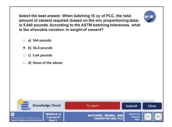
Select the best answer. When batching 10 cy of PCC, the total amount of cement required (based on the mix proportioning data) is 5,640 pounds. According to the ASTM batching tolerances, what is the allowable variation in weight of cement?
