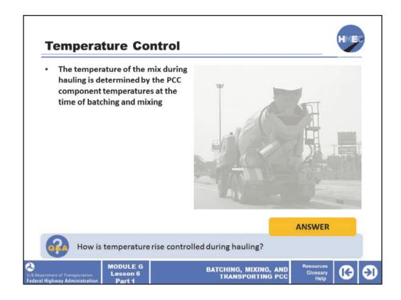
As was previously discussed, the temperature of the mix during hauling is determined by the PCC component temperatures at the time of batching and mixing.
