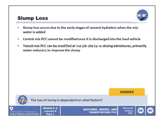
Slump loss occurs due to the early stages of cement hydration when the mix water is added. Central mix PCC cannot be modified once it is discharged into the haul vehicle. Therefore, the loss of slump must be anticipated during batching and mixing and adjustments made at that point. Transit mix PCC can be modified at the job site by redosing admixtures, primarily water reducers, to improve the slump.
