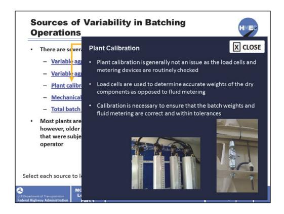
Plant calibration is generally not an issue as the load cells and metering devices are routinely checked.
