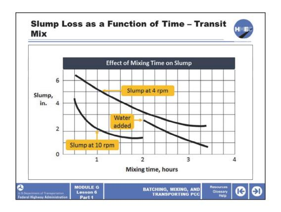
This slide illustrates general trends in slump loss. Unless retarding admixtures are used, slump loss will occur as a function of time, and in this case, mixing speed in the transit mixer.
