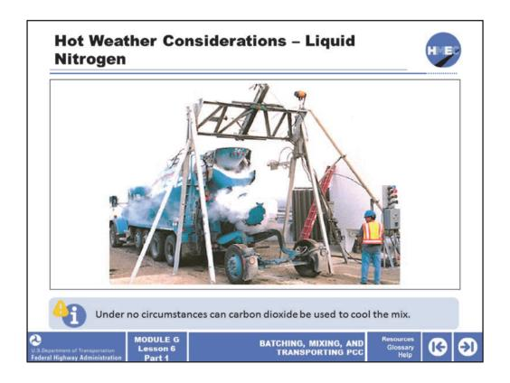
Liquid nitrogen may also be used under extreme temperature conditions to lower the temperature of the PCC mix. The photo shows liquid nitrogen being injected into the mixing drum of a transit mix truck. No adjustments to the mix proportions are required.
