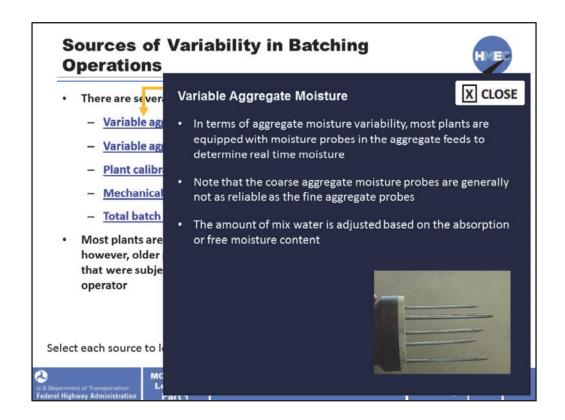
In terms of aggregate moisture variability, most plants are equipped with moisture probes in the aggregate feeds to determine real time moisture. Note that the coarse aggregate moisture probes are generally not as reliable as the fine aggregate probes.
