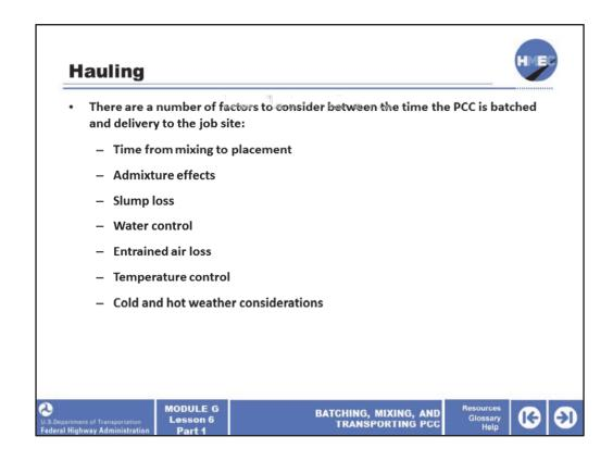
There are a number of factors to consider between the time the PCC is batched and delivery to the job site. Take a moment to read through the list on the slide.
