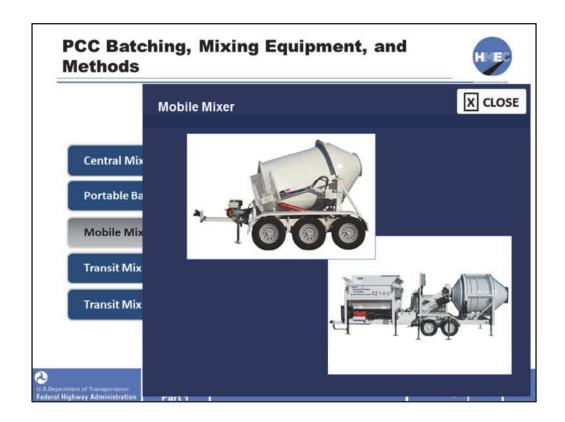
These photos show two types of mobile mixers. The unit on top is capable of producing 3 cy per batch, while the self-contained unit on the bottom can produce 1.3 cy of PCC per batch. These types of mixers are frequently used for patching and restoration projects where smaller batches are desired. In addition, they are used for difficult to reach or remote pours where a smaller volume of PCC is required.
