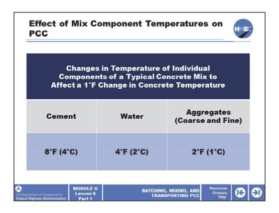
In order to facilitate a change in the PCC mix temperature of 1 °F, it would be necessary to lower the temperature of the cement by 8 °F, water by 4 °F, and aggregates by 2 °F.
