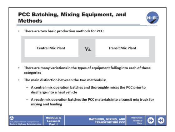
The manufacturing of PCC begins with the selection and processing of raw materials, a well proportioned mix based on intended use, and the selection of a production technique that matches the job requirements.
