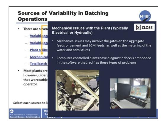
Mechanical issues may involve the gates on the aggregate feeds or cement and SCM feeds, as well as the metering of the water and admixtures.
