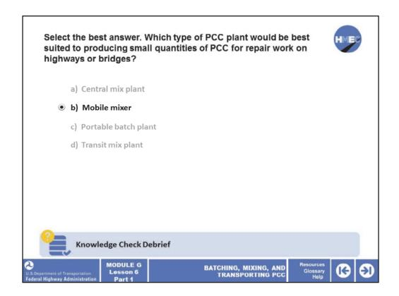
The correct answer is b) Mobile mixer. A mobile mixer is designed to produce small batches of PCC and would be ideally suited to this application.
