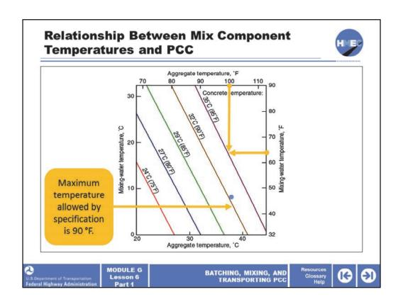
This slide illustrates the relationship between the primary components in PCC and mix temperature. For example, if the aggregate temperature is 100 °F and the water temperature is approximately 63 °F, the PCC temperature will be 95 °F.
