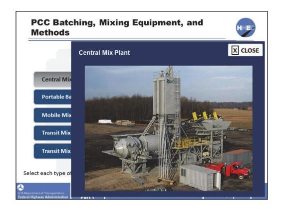
The photo shows a large "portable" central mix plant. Central mix plants typically produce approximately 100 to 600 cubic yards per hour depending on the plant configuration. For illustration, this plant is capable of producing up to approximately 550 cy of PCC per hour. The aggregate bins, cement, and supplementary cementing materials (SCM) silos, and the 12 cy mixing drum is visible in the photo.
