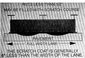
In instances where surface is uneven or where depth of wheel ruts is between 5 to 15 mm, two layers of microsurfacing may be used. The first application should be a scratch course to improve the transverse profile, followed by a surface course. This slide shows a spreader box with steel stake off and to fill shallow ruts.
