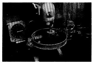
WTAT simulates wet abrasive conditions such as vehicle turning and breaking. In this test a cured sample 6 mm thick x 280 mm in diameter that has been soaked for an hour is immersed in a 25 °C water pan and is wet-abraded by a rotating weighted (2.3 kg) rubber hose for 5 minutes. The abraded sample is dried and weighed.
