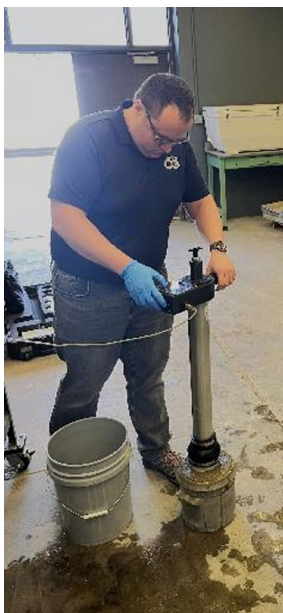
LEFT: Engineer Eric Desjardins uses the Instant Air Meter during a cooperative agreement demonstration event. RIGHT: Non-contact sensors measure real-time smoothness of freshly paved concrete during a demonstration. (Source: Concrete Pavement Technology Center)
