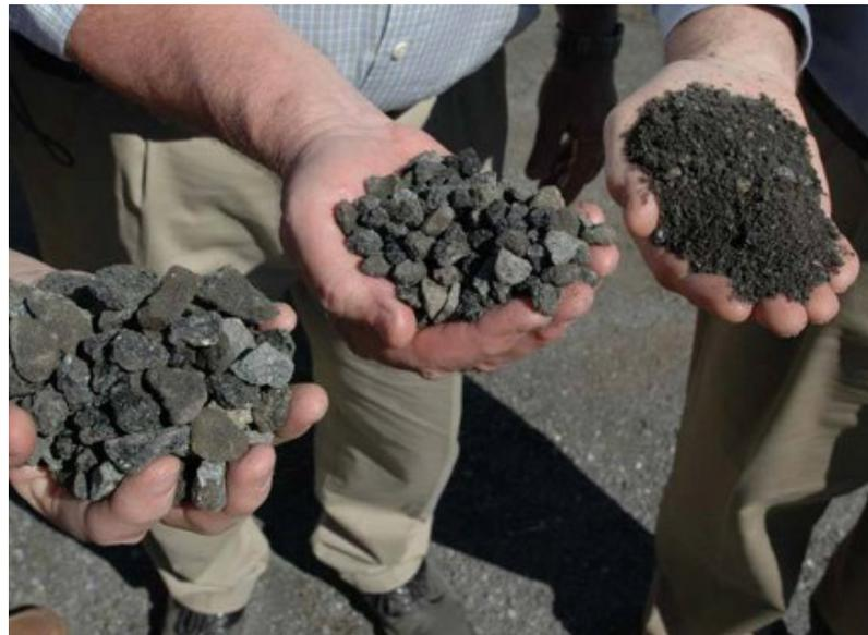
Using high-frequency screens and crushers to process RAP, crews can produce a variety of product sizes, which facilitates use in a wide range of applications. *Source: NCAT.*
