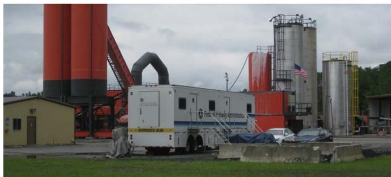
*FHWA's Mobile Asphalt Testing Trailer, shown here at a plant in Lake City, FL, recently visited projects in Florida and Arizona to evaluate the performance of GTR. The mobile testing trailer also supported the American Association of State Highway and Transportation Officials and ASTM International in revising the standards for evaluating binders incorporating GTR.*
