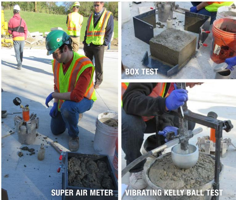
Innovative tests represented in the new specification for concrete pavements. Source: National Concrete Pavement Technology Center.
