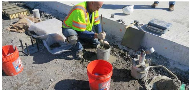
A technician from the Mobile Concrete Trailer is preparing a fresh concrete sample for air void testing at a project site. Source: APTech.
