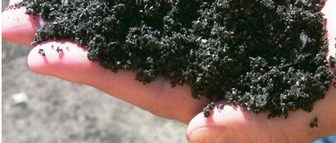
This handful of processed shingles, or RAS, is ready for inclusion in an asphalt mixture.
