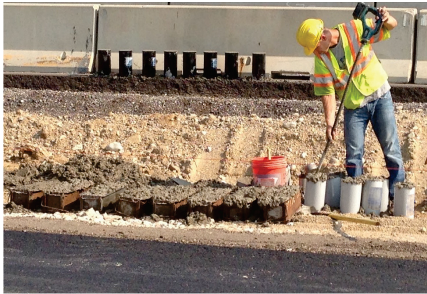
Figure 31. Preparing beams and cylinders on Illinois Tollway PCC/PCC project.
