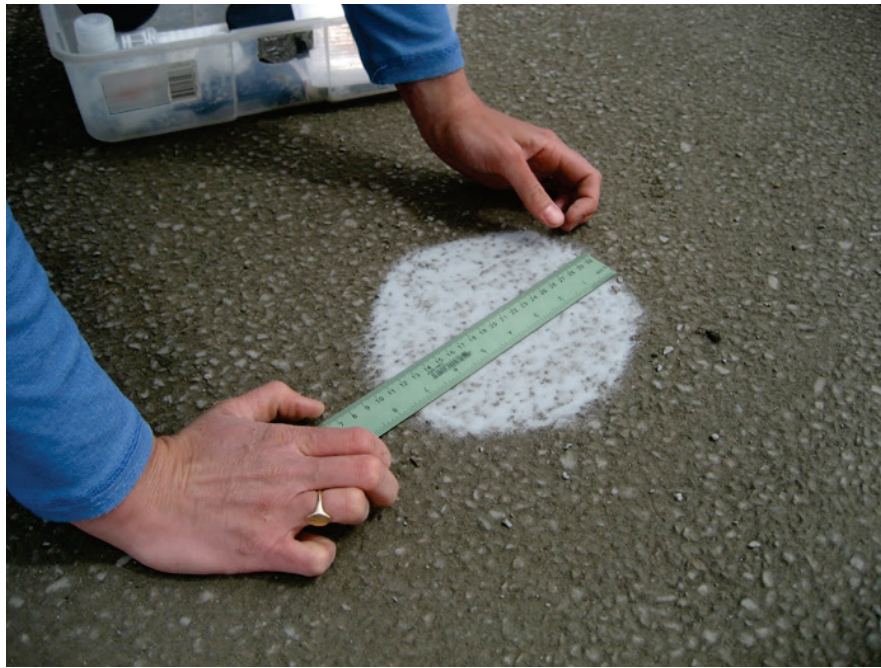
Figure 38. Measuring mean texture depth on exposed aggregate surface on Mn/Road PCC/PCC composite pavement.
