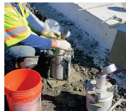
c) Air test (left: Super Air Meter, right: standard air meter)
