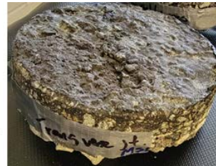
Figure 1. An LTS scan of a field core with microsurfacing treatment and an image of the original core. Source: NCDOT.
