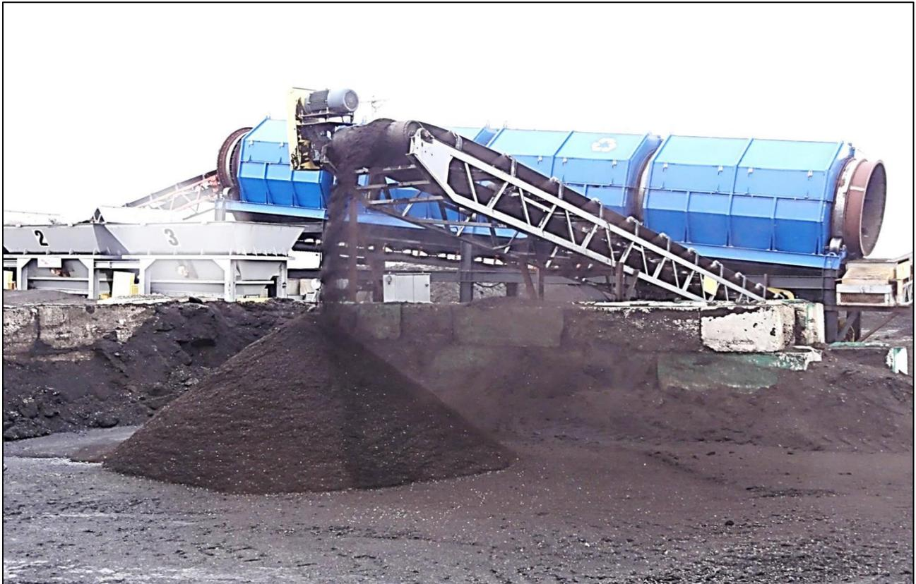
Photo of a trommel, a rotary screen, sizing reclaimed asphalt shingles.
