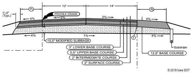
Figure 2. Iowa 100 pavement cross section design.
