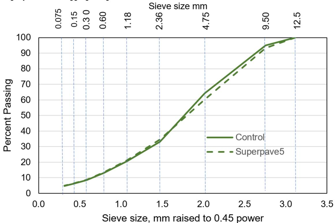
Figure 1. Asphalt-concrete aggregate gradations for control and Superpave5 used at the U.S. 40 project.
