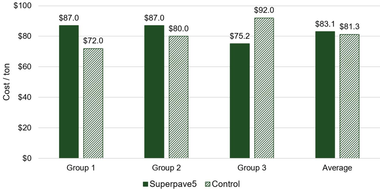
Figure 2. Cost comparison of the production of Superpave5 and control mixes.
